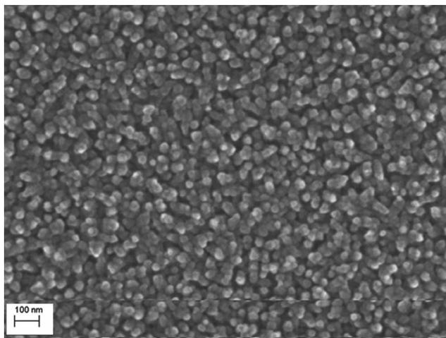
**Figure 3** | AFM image of the silver-coated ceramic surface where the diameters of the nano-particles vary between 40 and 50 nm.**Table 3** | Oligodynamic action of silver-coated ceramic
