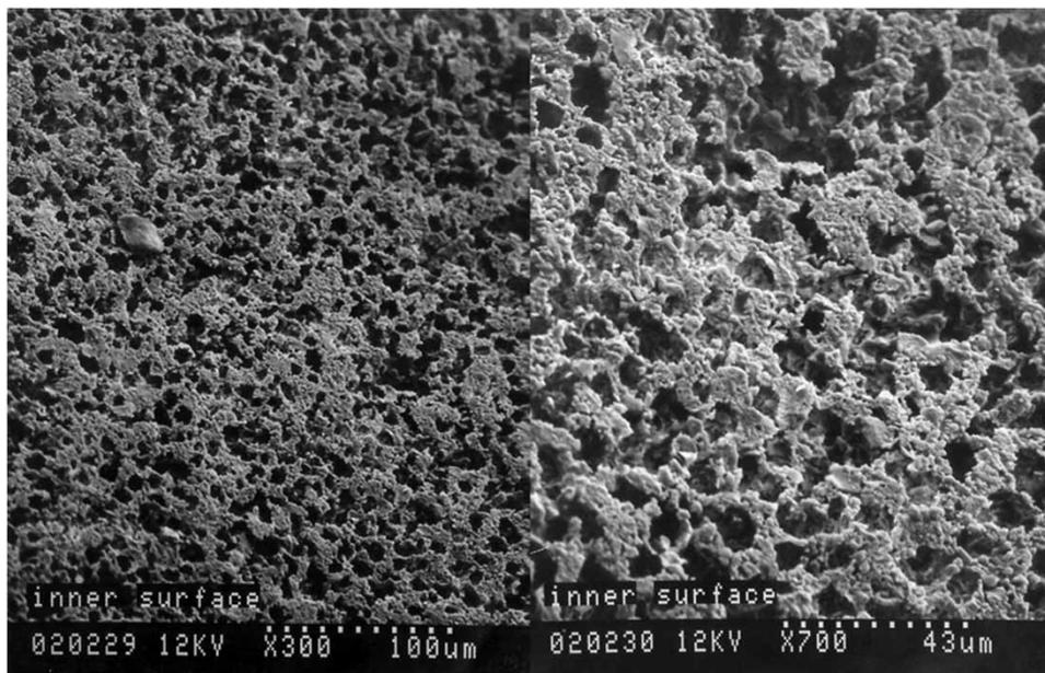
**Figure 2** | SEM images of the OUTBAC filter surface showing the homogeneous pore size distributions of the larger and smaller pores with  $d_{50}$  (average pore size) of 5 and 0.3 micron, respectively.
