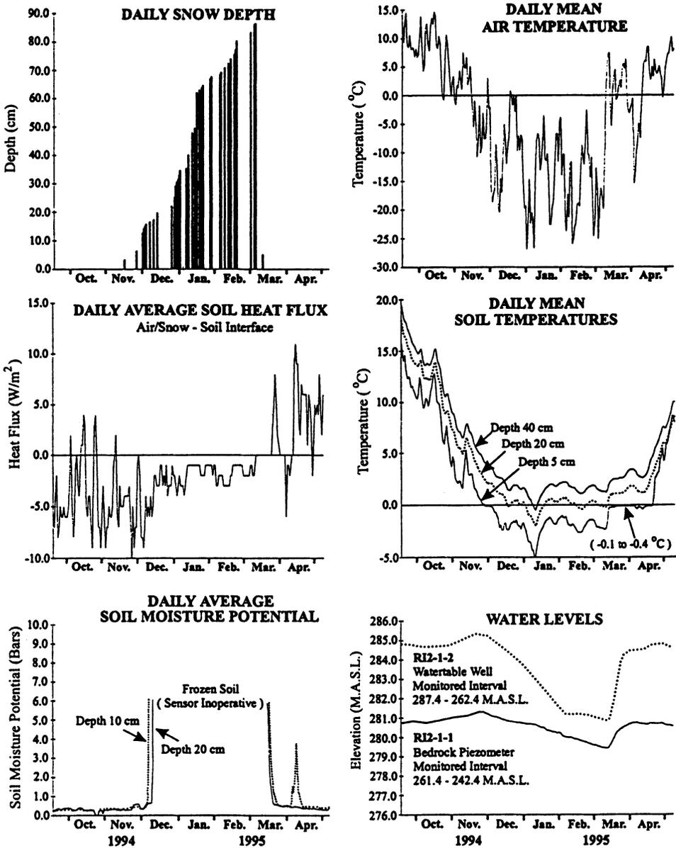
Fig. 3. Snow depth, air and soil temperatures, soil heat flux, soil moisture potential and water levels for the outcrop groundwater recharge area.
