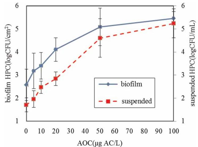
Figure 5 | Relationship of AOC and average steady-state HPC.
