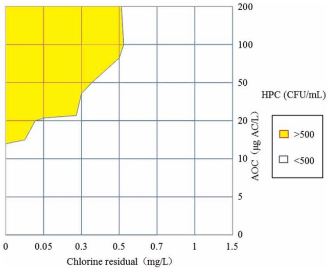
**Figure 6** | Impact of AOC and chlorine residual on the suspended HPC of the distribution system.
