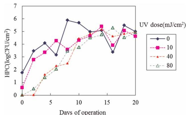
Figure 3 | Impact of UV doses on biofilm HPC in the distribution system.
