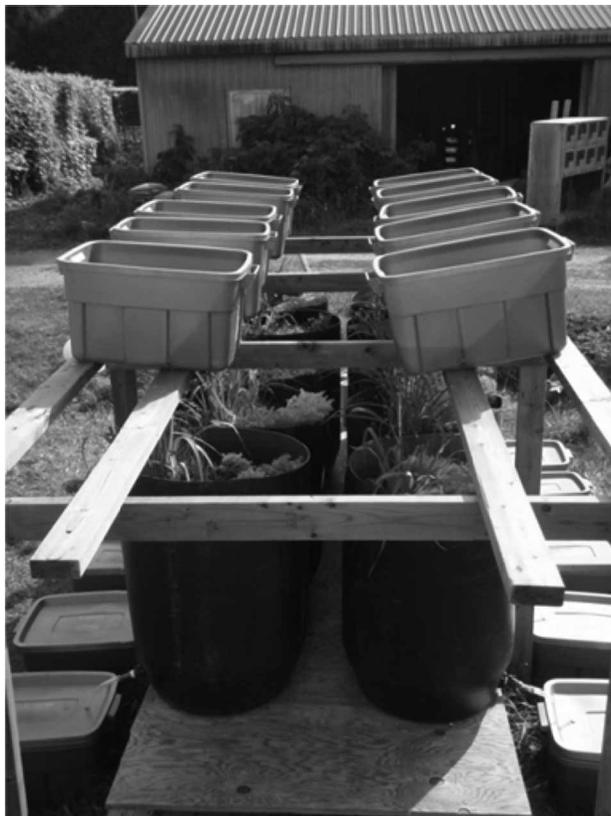
**Figure 1** | Photograph of constructed bioretention mesocosms.
