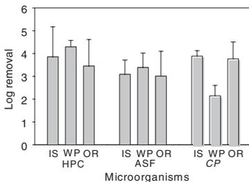
**Figure 4** Total log removal of microorganisms through water treatment process
