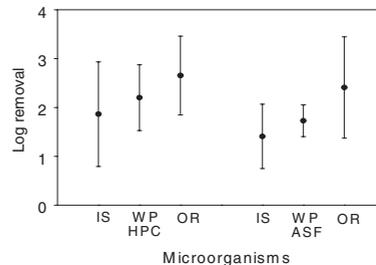
**Figure 5** Log removal of microorganisms in coagulation and sedimentation
