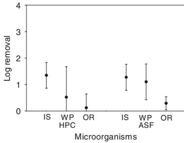
**Figure 6** Log removal of microorganisms in filtration step
