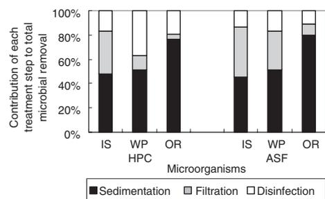
**Figure 9** Contribution of each treatment step to total microbial removal in water treatment plants
