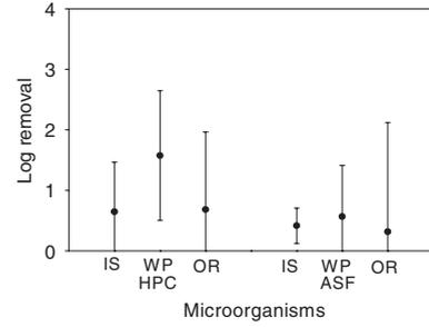
**Figure 7** Log removal of microorganisms in disinfection step
