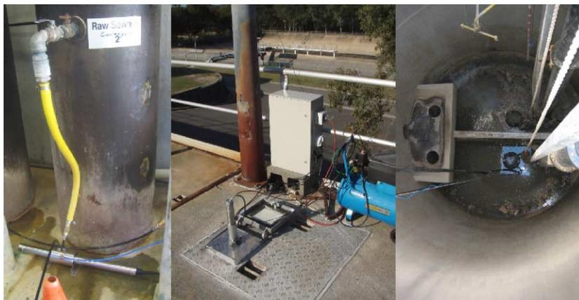
**Figure 2** | Deployment of the spectrometer. Site 1: in a bypass fitting, Site 2: installed in a sealed box channel and Site 3: hidden from view at the bottom of a wet well.
