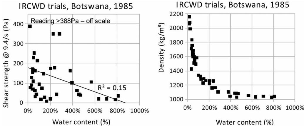
Figure 1 | Effect of water content on sludge properties.
