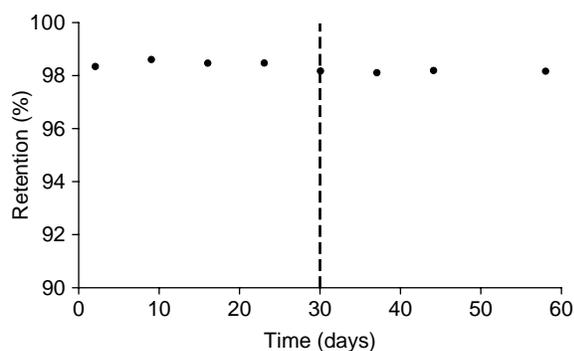
**Figure 3** | Retention based on conductivity with time for the membrane element operated with periodic air/water cleaning (twice per week) under permeation conditions. The dashed line indicates the start of the periodic air/water cleaning.
