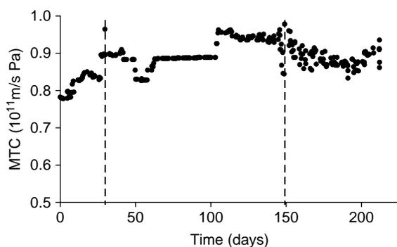
**Figure 2** | Membrane transport coefficient (MTC) with time for the membrane element operated with periodic air/water cleaning (twice per week) under permeation conditions. The dashed lines indicate (left) the start of the periodic air/water cleaning and (right) the extensive cleaning of the feed vessel.
