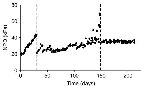
**Figure 1** | Normalized pressure drop (NPD) with time for the membrane element operated with periodic air/water cleaning (twice per week) under permeation conditions. The dashed lines indicate (left) the start of the periodic air/water cleaning and (right) the extensive cleaning of the feed vessel.
