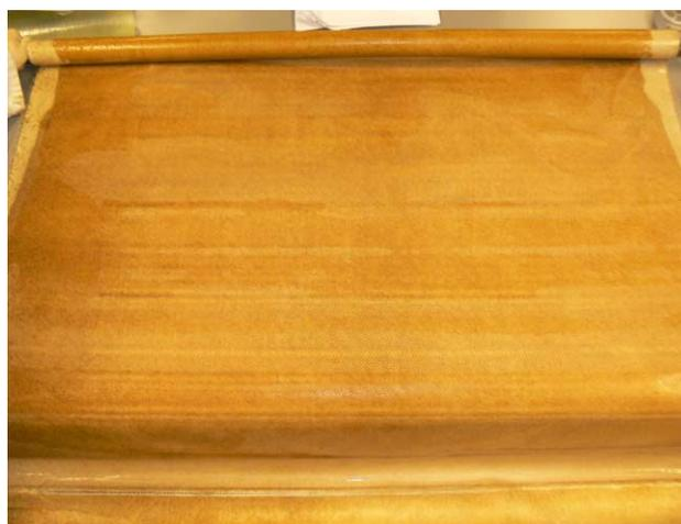
**Figure 4** | Fouled membrane sheet from the membrane element operated under permeation conditions with AWC after 212 days. The flow direction was from right to left.
