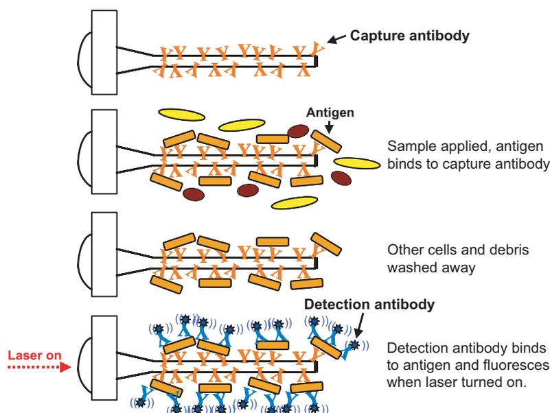
**Figure 3** | Biosensor sandwich assay. Target antigen is bound by a capture antibody on the fiber optic waveguide. A fluorophore (Cy5)-labeled detection antibody is then attached to form a sandwich assay. The fluorophore is excited by a laser to generate a detectable signal.
