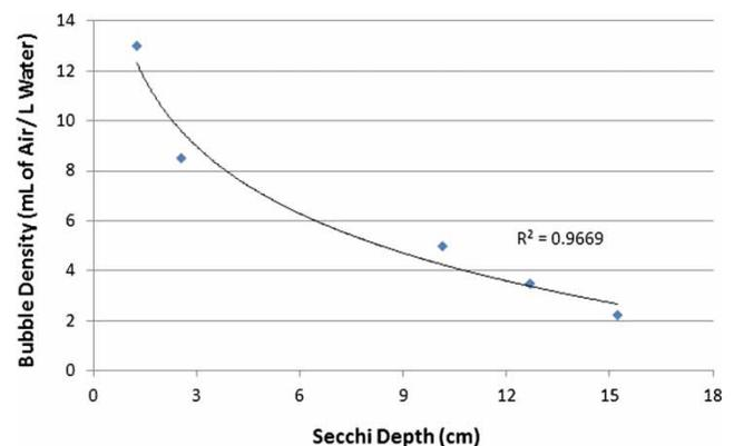
**Figure 4** | Calibration between Secchi depth and bubble density generated using ambient air in freshwater at room temperature (c. 23 °C).
