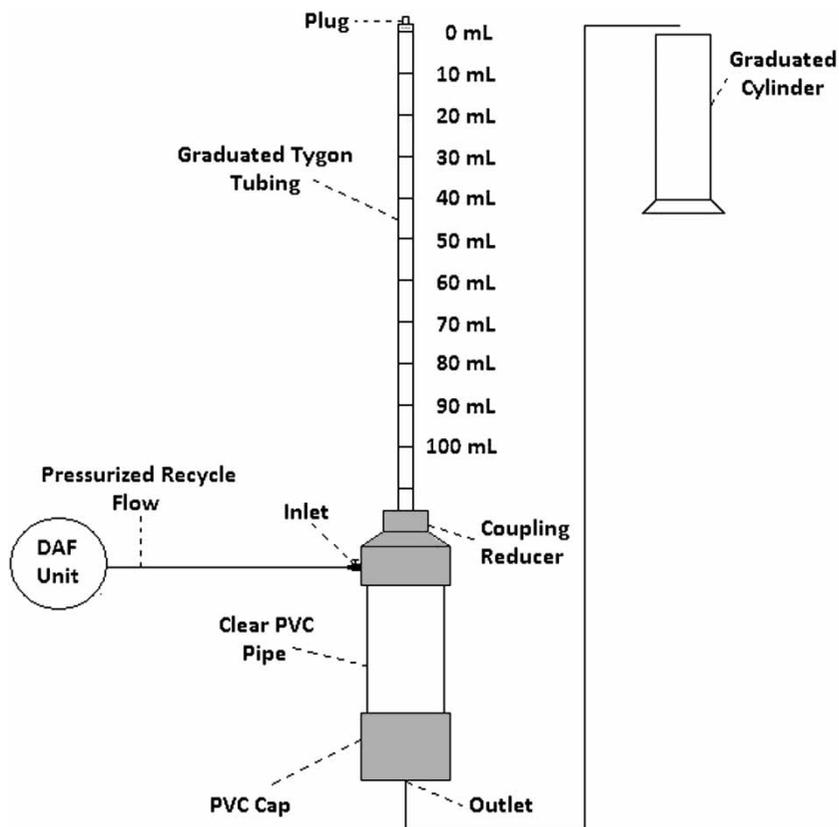
**Figure 1** | An in-house-built air quantification unit was used to quantify the air released after depressurization. This unit can be effectively used for optimization of DAF treatment systems.
