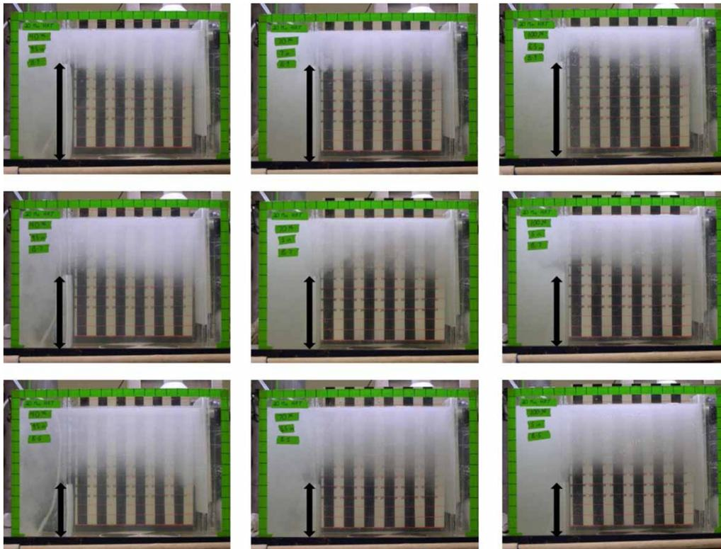
**Figure 3** | Photographs depicting the bubble density patterns inside the flotation tank for various baffle heights and recycle ratios. The images were taken when the black-and-white edges of the grids were distinctly visible. The corresponding depths of the grids are listed in Table 1. The saturated flow was released to the left of the baffle at the bottom of the tank. Baffle heights are shown by superimposed double arrows.
