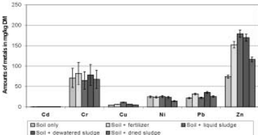
**Figure 3** Amounts of metal trace elements in the amendments-soil mixtures
