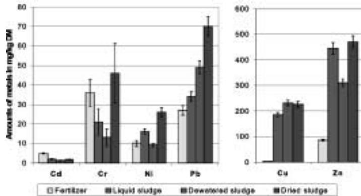
**Figure 2** Amounts of metal trace elements in the amendments
