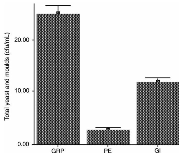
**Figure 7** | TC of yeast and moulds of GRP, PE and GI tanks ( $n = 40$  replications/treatment).
