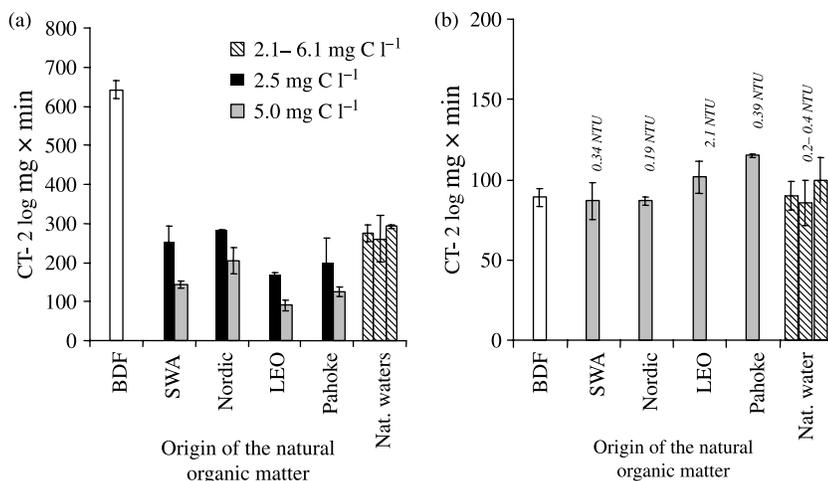
**Figure 3** | Values of Ct (2log) for inactivation of *B. subtilis* spores using chlorine dioxide (a) or free chlorine (b) for several synthetic and natural waters. BDF water (buffered demand-free) represents the reference. Error bars represent the 95th percentile confidence interval. T:  $22^\circ\text{C}$ , pH 6.5.
