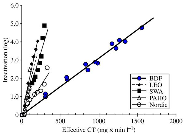
**Figure 1** | Inactivation of *B. subtilis* spores using chlorine dioxide for several synthetic waters ( $5 \text{ mg Cl}^{-1}$ ). BDF (buffered demand-free) represents the reference condition. Bold lines provide the Chick-Watson kinetics. T:  $22^\circ\text{C}$ , pH 6.5.
