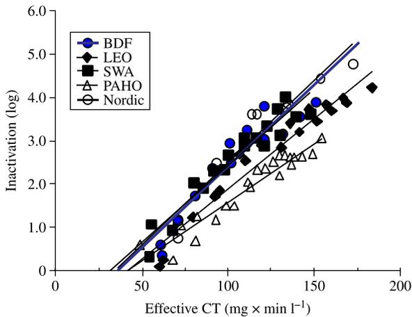
**Figure 2** | Inactivation of *B. subtilis* spores using free chlorine for several synthetic waters ( $5 \text{ mg Cl}^{-1}$ ). BDF water (buffered demand-free) represents the reference condition. Bold lines provide delayed Chick-Watson kinetics. T:  $22^\circ\text{C}$ , pH 6.5.
