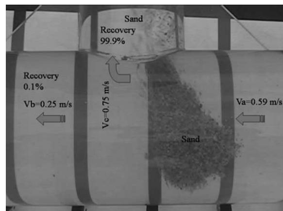
Figure 5 | Experiment on T branch ( $\varphi 150 \times \varphi 100$ ).
