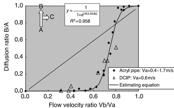
Figure 4 | Diffusion ratio at branch Sand in T branch  $\varphi 150 \times \varphi 100$ .
