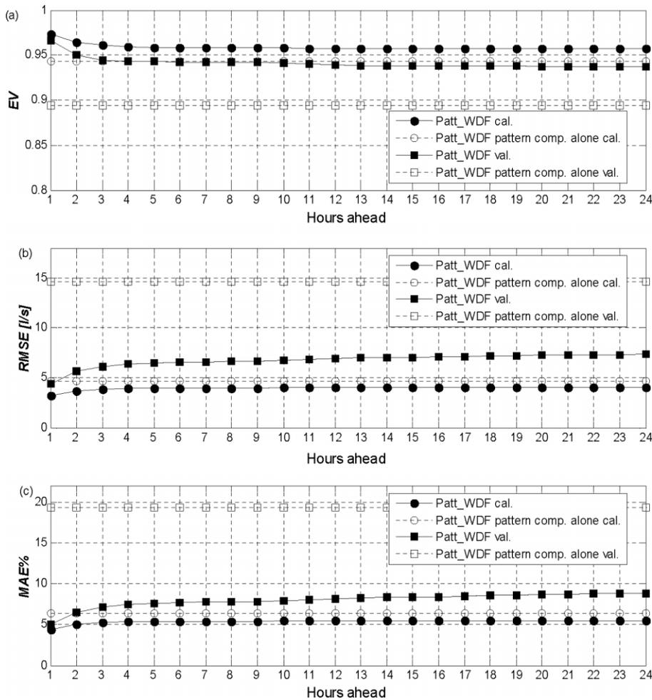
**Figure 8** | EV, RMSE and MAE% between the observed hourly water demands and those forecast with the Patt\_WDF model, based on the periodic component alone and on the complete model, 1, 2, ..., 24 h ahead in the calibration (cal.) and validation (val.) phases.
