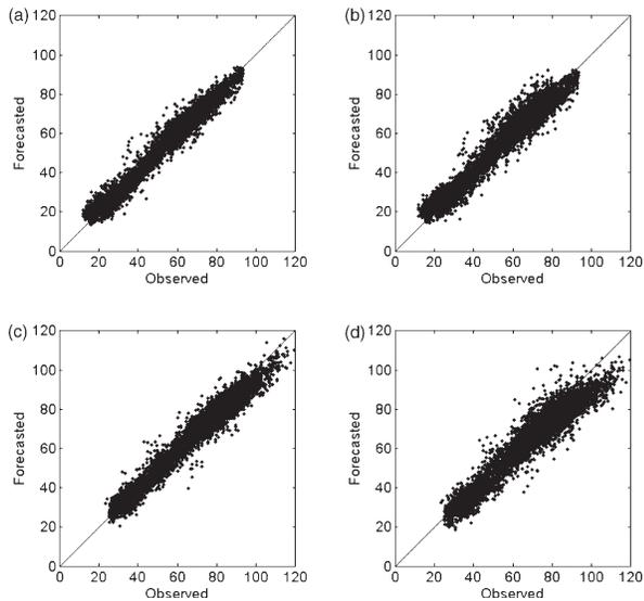
**Figure 9** | Water demand as forecast (a) 1 h ahead in the calibration phase, (b) 24 h ahead in the calibration phase, (c) 1 h ahead in the validation phase and (d) 24 h ahead in the validation phase, compared to the observed data.
