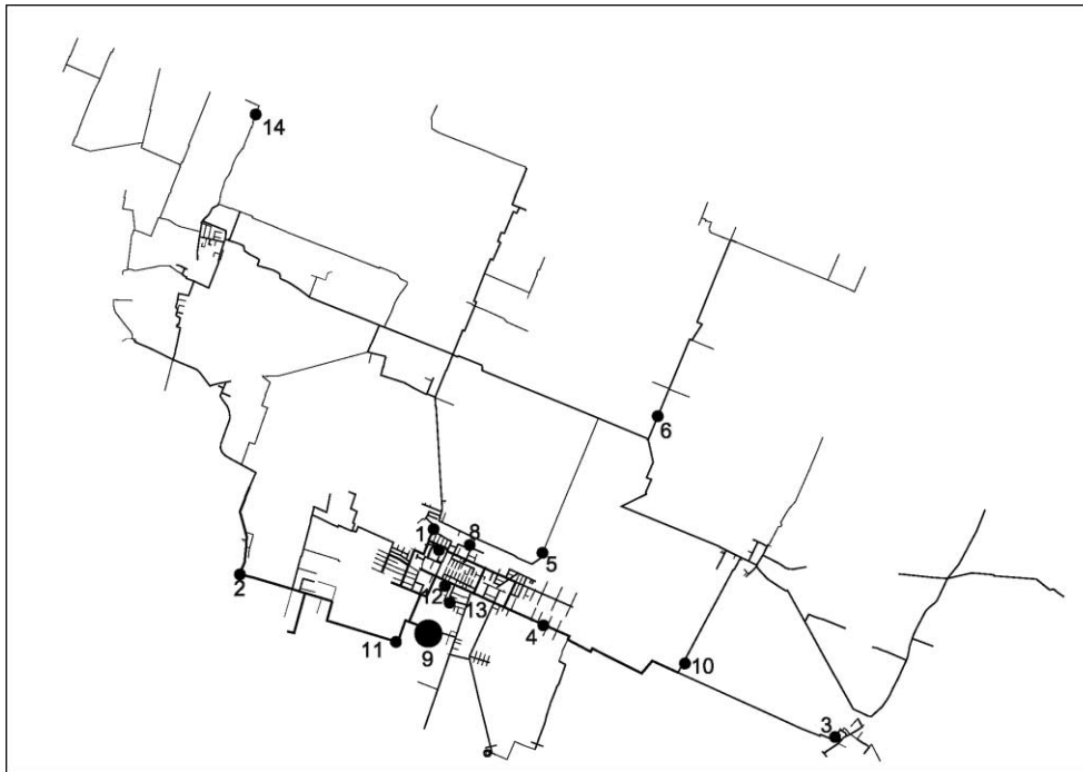
Figure 1 | The main water distribution network of Castelfranco Emilia (Province of Modena, Italy) and location of the 14 monitoring stations installed. Station 9 was used in this study.
