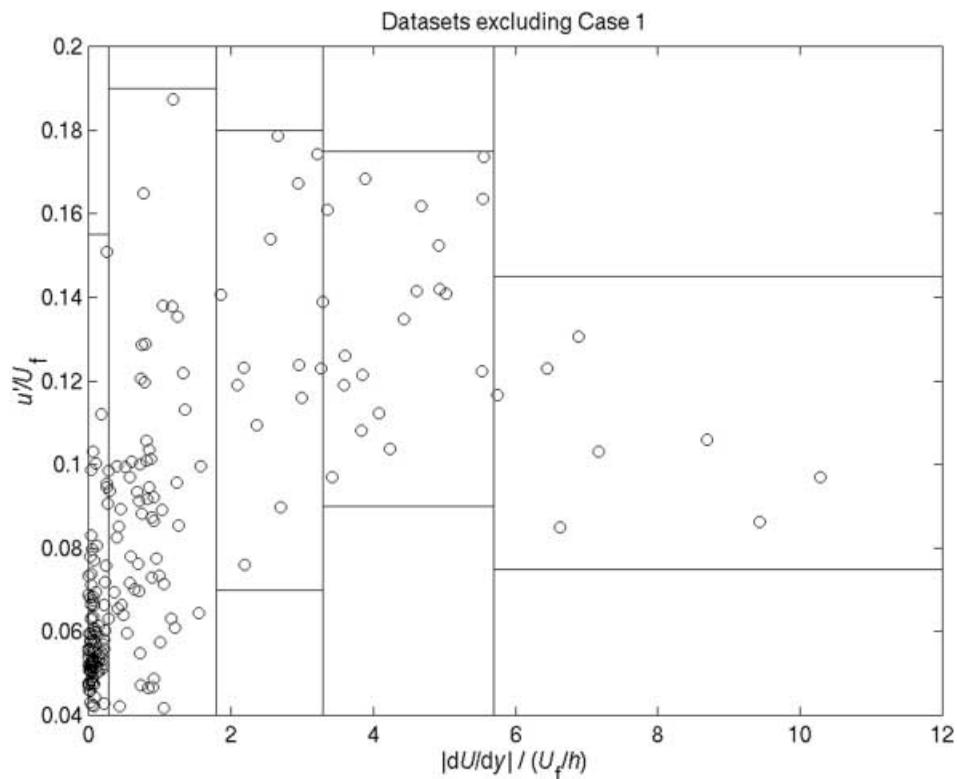
**Figure 5** | Non-dimensionalized distribution of  $u'$  against non-dimensionalized transverse velocity shear. Straight lines show support of membership functions to be used in the fuzzy inference system.
