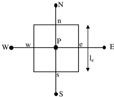
Figure 10 | A control volume around node P.
