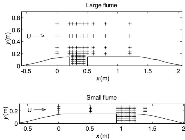
**Figure 1** | Plan view of experimental conditions showing velocity data collection points, +, in large and small flumes.
