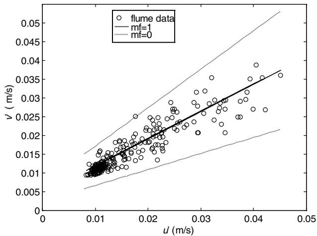
**Figure 7** | Fuzzy regression for cross stream and longitudinal velocity fluctuations with  $v'$  shown as a fuzzy number whose most likely value is shown by the line where the membership function (mf) is one. The support of the fuzzy number is defined by the zero membership lines.
