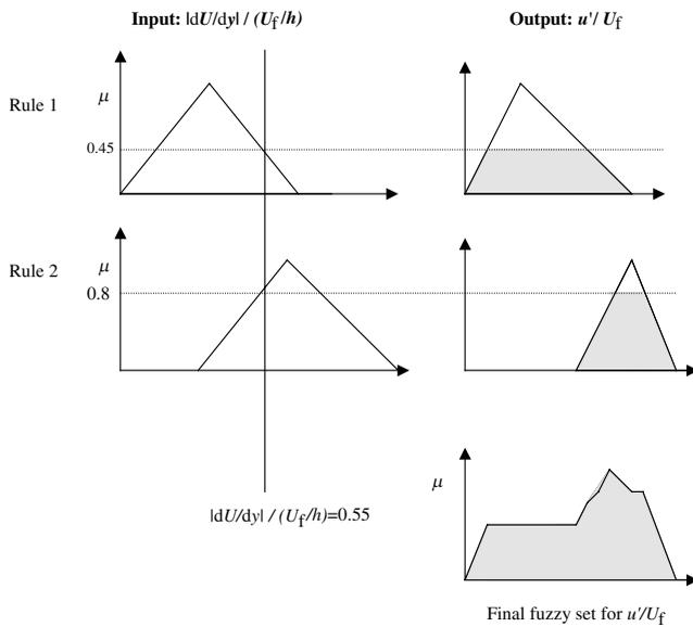
**Figure 4** | A simplified example of how a fuzzy inference system uses a value for the non-dimensionalized transverse velocity shear in 2 rules to produce 2 fuzzy sets for the non-dimensionalized velocity fluctuation. These rule responses are then aggregated using the sum method to produce a single fuzzy set.
