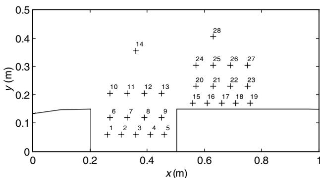
Figure 12 | Location and numbering of thermocouples.
