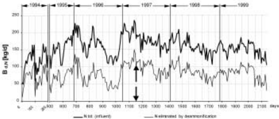
Figure 4 Presentation of influent and eliminated nitrogen loads in the RBC plant of Mechernich
