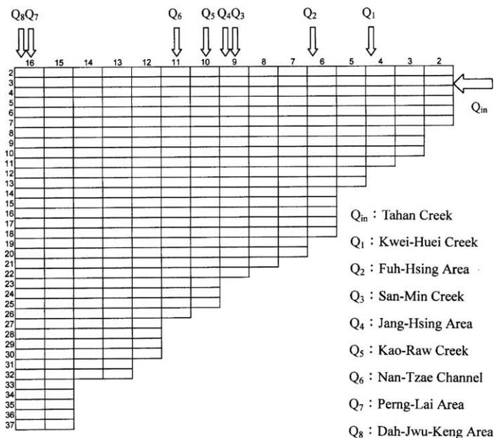
**Figure 5** Finite different grid representation for the model of the Shihmen Reservoir
