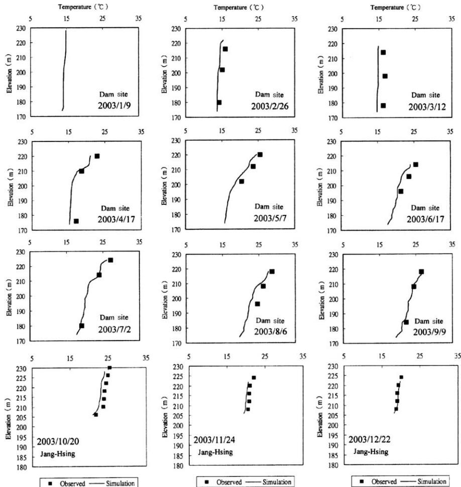
**Figure 7** Predicted and observed water temperature for 2003 calibration
