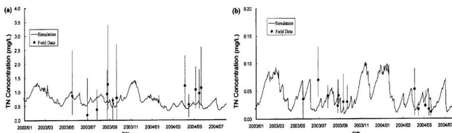
**Figure 4** The comparisons of model results and field data from 2003 to 2004 (a) total nitrogen and (b) total phosphorus concentrations
