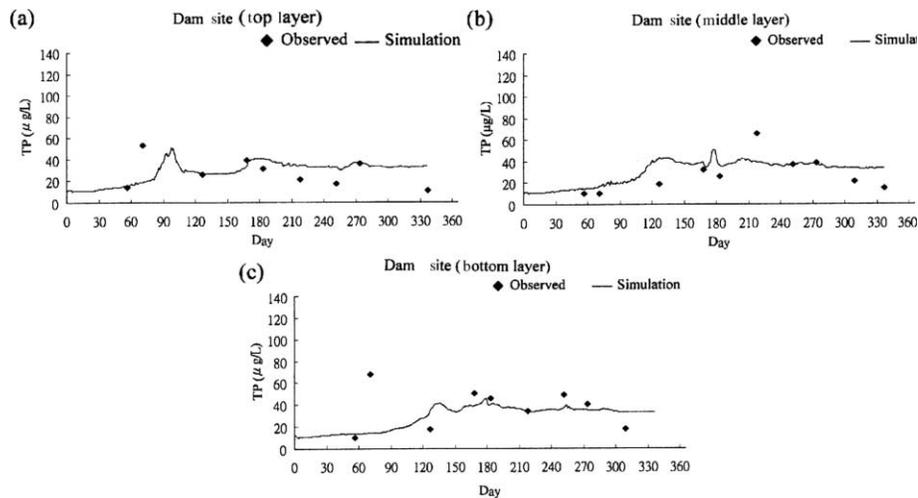
**Figure 9** Predicted and observed total phosphorus concentration for 2003 model calibration at dam site (a) surface layer, (b) middle layer, and (c) bottom layer
