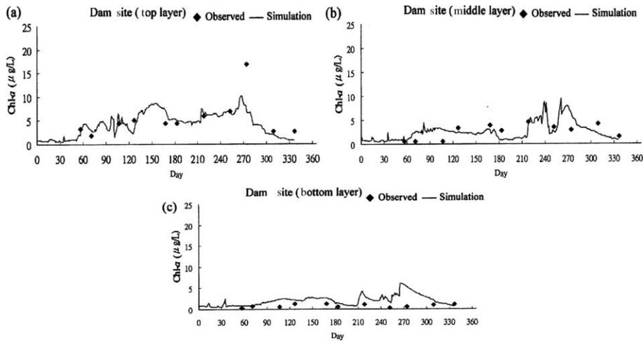
**Figure 8** Predicted and observed chlorophyll a concentration for 2003 model calibration at dam site (a) surface layer, (b) middle layer, and (c) bottom layer
