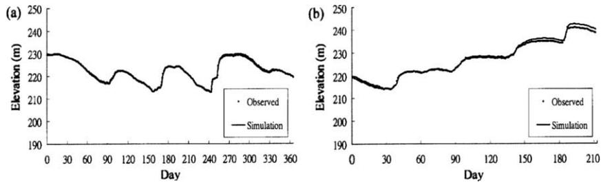
**Figure 6** Water surface elevation of model simulation vs. field data (a) 2003 and (b) 2004
