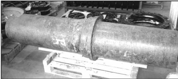
**Figure 1** | The outside surface of cast iron for water supply pipe constructed in 1887 in Yokohama City.
