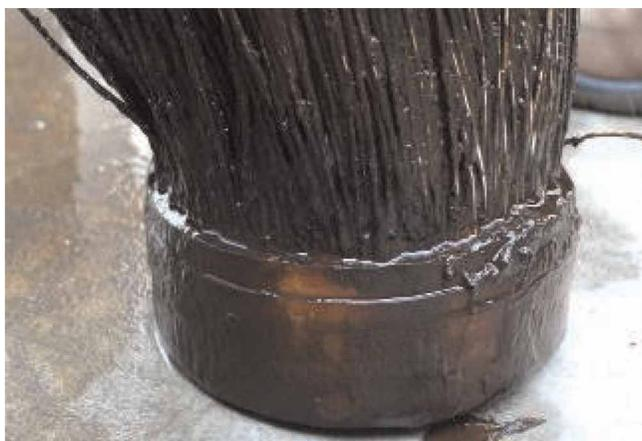
**Figure 7** | The formation of Fe–Mn sludge on the PTFE membrane.
