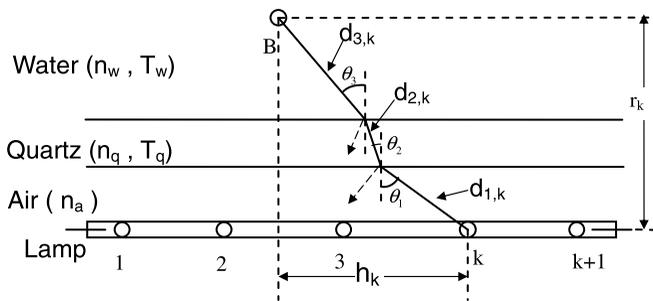
Figure 3 | Illustration of the attenuation factor calculation.
