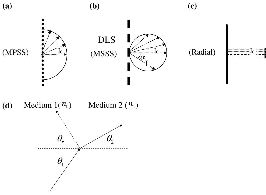
**Figure 1** | Fluence rate production with (a) MPSS, (b) DLS or MSSS and (c) radial approaches, (d) refraction and reflection at the interface of two media with different refractive indices.
