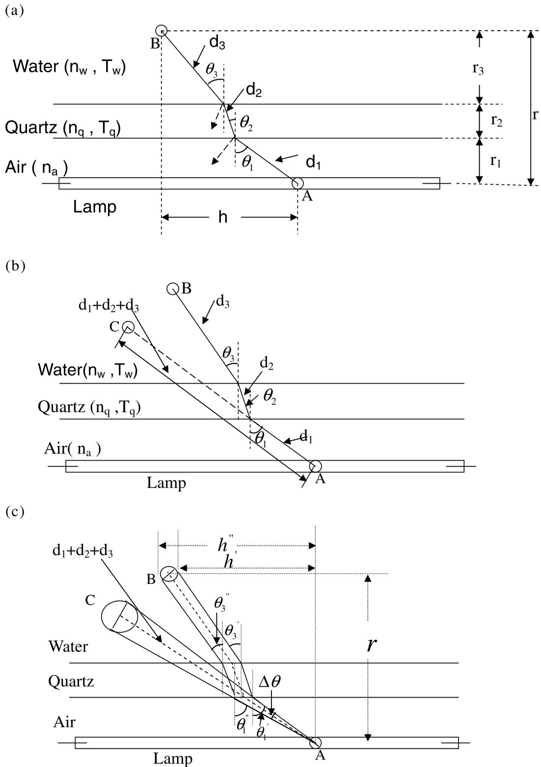
**Figure 2** | Components of refraction: (a) refraction angle calculation, (b) bending effect and (c) focus effect.
