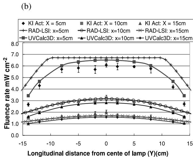
**Figure 7** | Fluence rate distribution along the lamp at different normal distance to the lamp ( $x=5, 10, 15$  cm): (a) impact of LSI, (b) impact of RAD-LSI.
