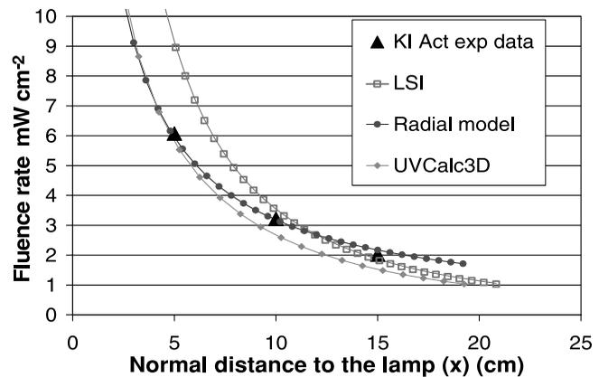
**Figure 8** | Fluence rate radial distribution on the profile of the centre point of the lamp.
