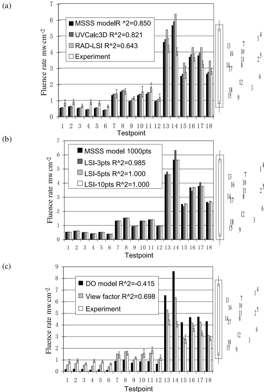
**Figure 9** | Fluence rate value in water at test points: (a) comparison between UV Calc3D, RAD-LSI and MSSS models, (b) determination of appropriate  $n$  value for attenuation factor, (c) comparison between DO and view factor models.
