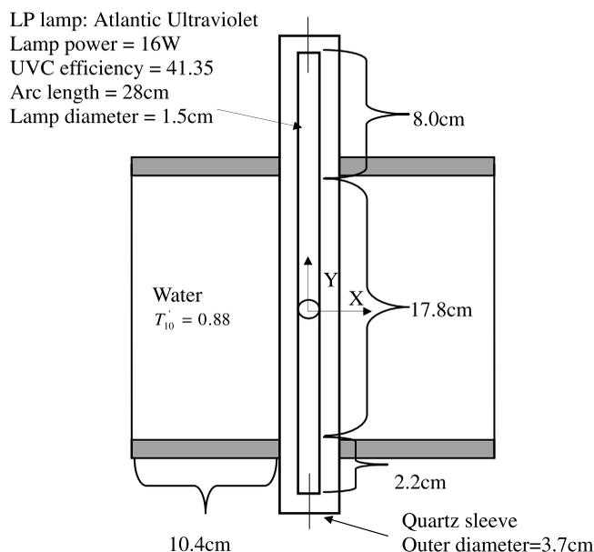
**Figure 6** | Nickel plated stainless steel reactor filled with water for transmissivity tests.
