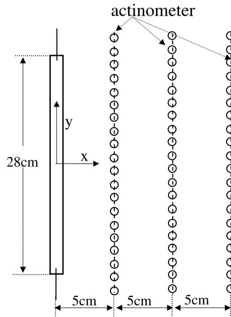
Figure 5 | Schematic illustration of test reactor in the air.
