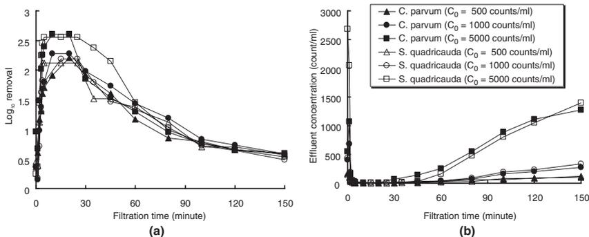
**Figure 3** (a) The removal rates and (b) effluent levels of *S. quadricauda* and *Cryptosporidium* for the initial levels of 500, 1,000 and 5,000 counts per ml
