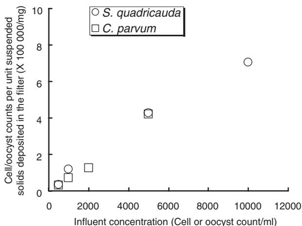
**Figure 5** Relationship between the initial levels and the cell/oocyst counts per unit suspended solids deposited in the filter
