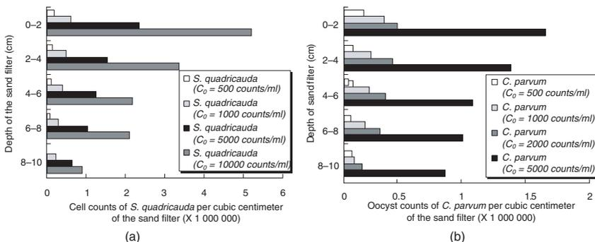
**Figure 4** The counts of: (a) *S. quadricauda* and (b) *C. parvum* oocysts deposited in the unit volume (1 cm<sup>3</sup>) of the sand filter (total filter volume is about 70 cm<sup>3</sup>)
