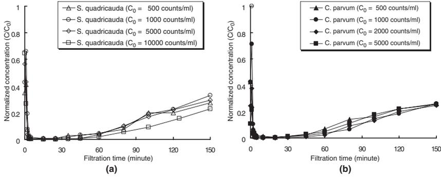
**Figure 2** The effluent concentration profiles ( $C/C_0$ ) of: (a) *S. quadricauda*, and (b) *C. parvum* oocysts for various initial levels
