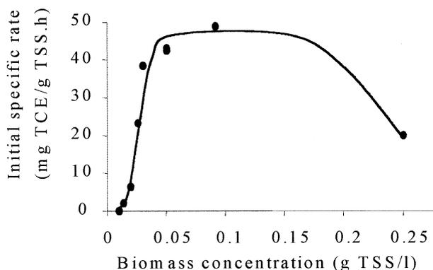
**Figure 7** Initial specific TCE degradation rate versus biomass concentration for consortium B
