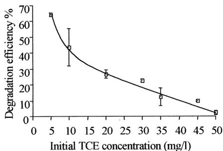
**Figure 3** Degradation efficiency versus initial TCE concentration on consortium C
