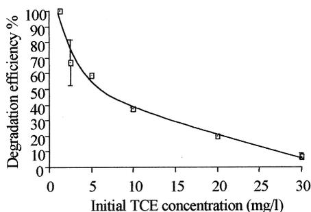
**Figure 2** Degradation efficiency versus initial TCE concentration on consortium B
