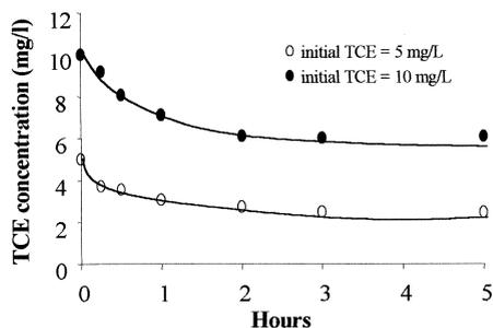
**Figure 4** TCE concentration versus time for initial TCE concentration of 5 and 10 mg/l, with Consortium B (TSS=250 mg/l)
