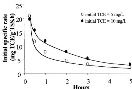
**Figure 5** Initial specific TCE degradation rate versus time for initial TCE concentration of 5 and 10 mg/l, with Consortium B (TSS = 250 mg/l)
