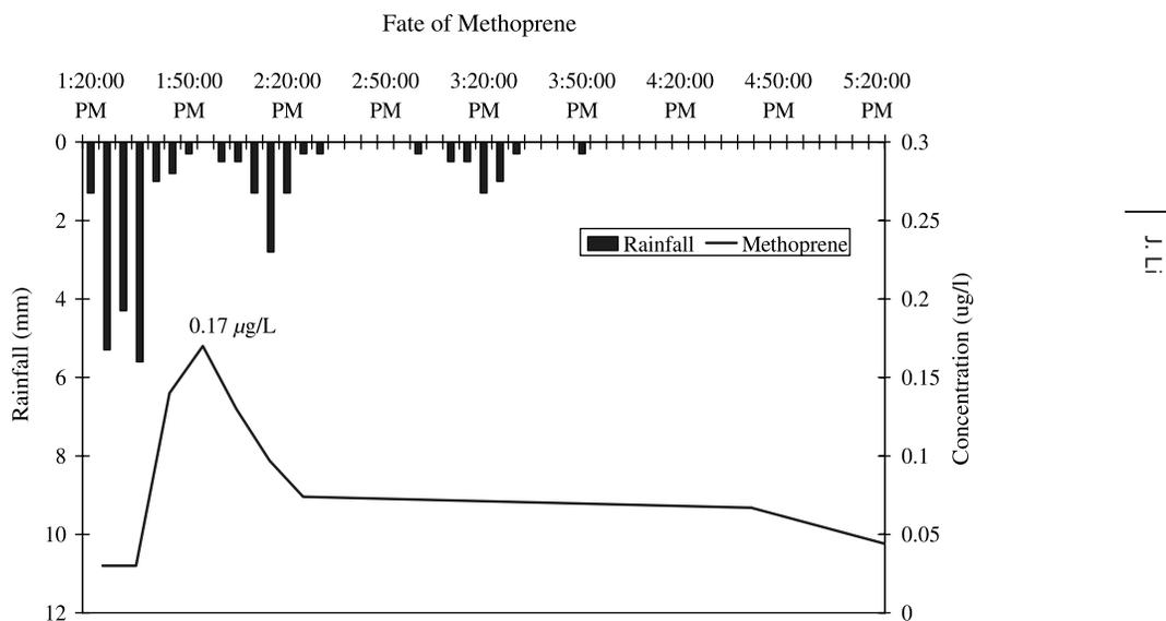
**Figure 2** Methoprene concentration at the sewer outfall during a rain storm
