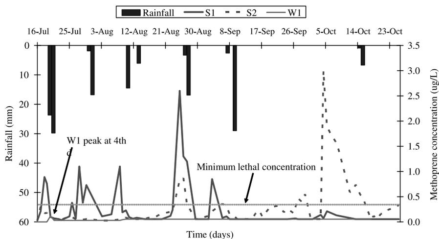
Figure 1 Residual methoprene concentration at catch basins
