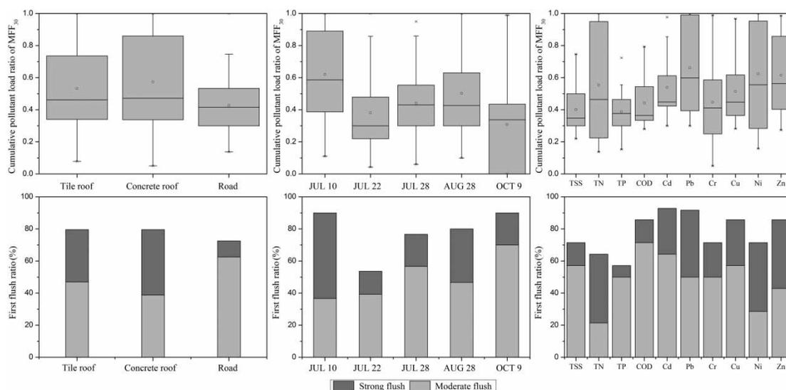
**Figure 4** | The MFF<sub>30</sub> cumulative pollutant load and FF probability of different sampling sites, rainfall events and pollutants. Moderate flush:  $1 < \text{MFF}_{30} < 2$ ; strong flush:  $\text{MFF}_{30} \geq 2$ . FF ratio refers to the moderate and strong flush events as a proportion of the total event.
