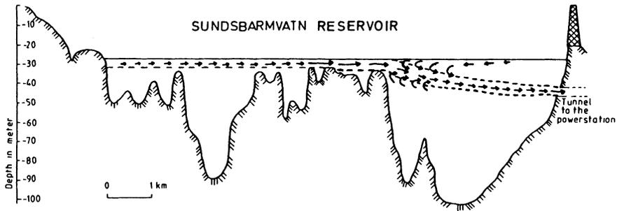
Fig. 6. The flow pattern in Sundsbarmvatn Reservoir at the end of the winter period as interpreted from the temperature measurements
