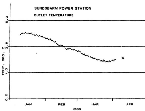
Fig. 4. The temperature at the outlet tunnel from the Sundsbarm Power Station from 10 Jan. to 11 April 1985. The temperature is recorded every fourth hours.
