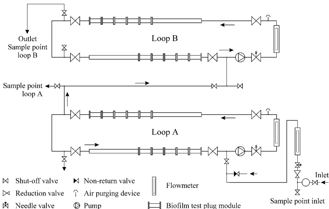
Figure 1 | The model distribution system.
