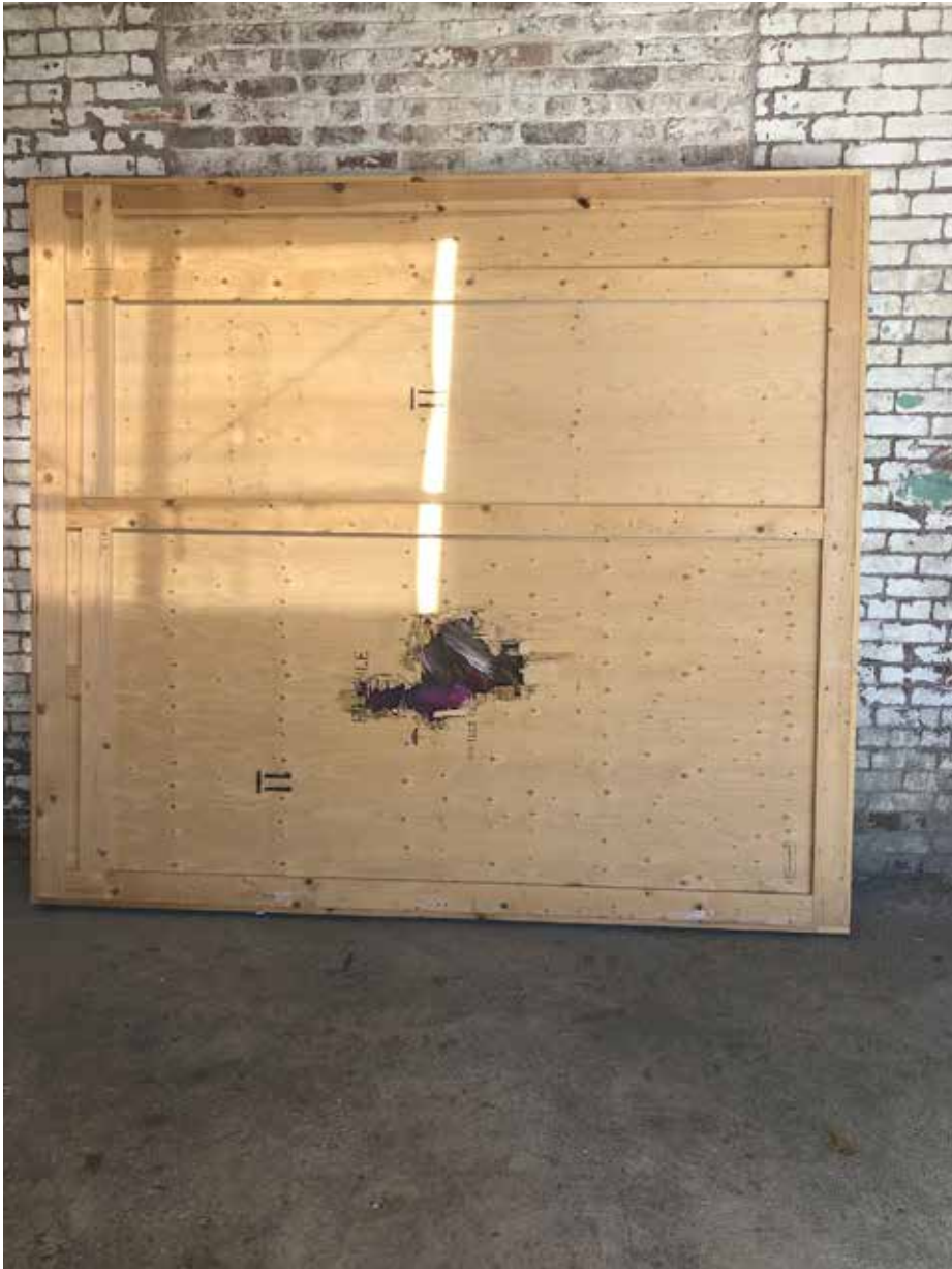
FIGURE 2. Ruptured wooden shipping crate. Photograph by author.
