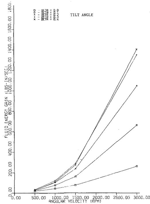
Fig. 18 Fluid energy gain in a hydrodynamic bearing under adiabatic conditions ( $R = 1.5$  m,  $c = 0.003$  in.)
