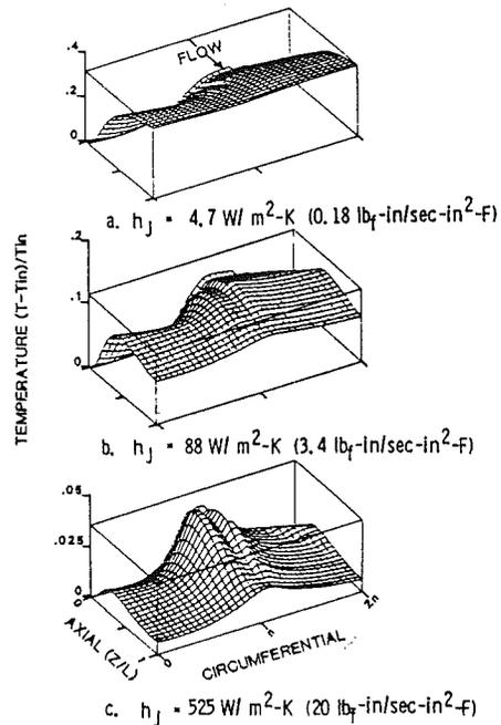
Fig. 16(a) Variation of axial and circumferential temperature profile with changes in heat transfer coefficient to the journal for a tilt angle of  $0.4$   $T_{in} = 38$  C and rpm = 1000
