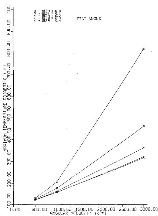
Fig. 17 Maximum temperature in a hydrodynamic bearing under adiabatic conditions (radius = 1.5 in. radial clearance  $c = 0.003$  in.)
