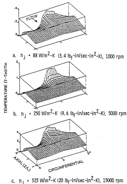
Fig. 16(b) Variation of axial and circumferential temperature profile with angular velocity and heat transfer coefficient to the journal for a tilt angle of  $0.48$ ,  $T_{in} = 38$  C
