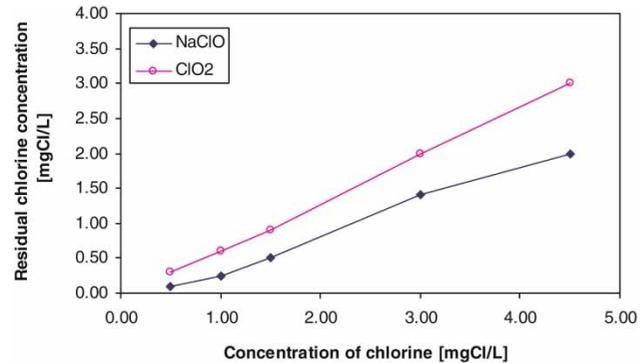
**Figure 3** | Residual chlorine after MC-LR oxidation with sodium hypochlorite and chlorine dioxide.
