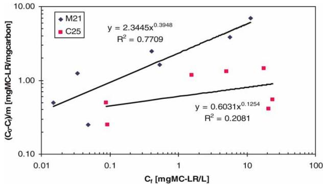
Figure 5 | Activated carbon sorption isotherm for MC-LR.
