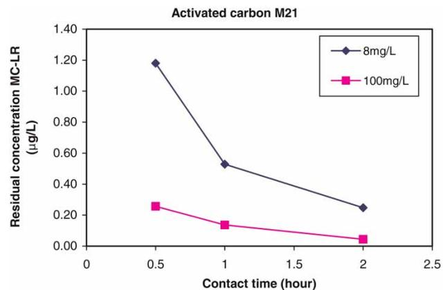
**Figure 4** | Residual concentration of MC-LR versus different contact times with activated carbon M21.
