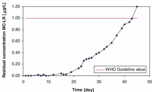
Figure 6 | Residual concentration of MC-LR in treated water during column test filtration with activated carbon M21.
