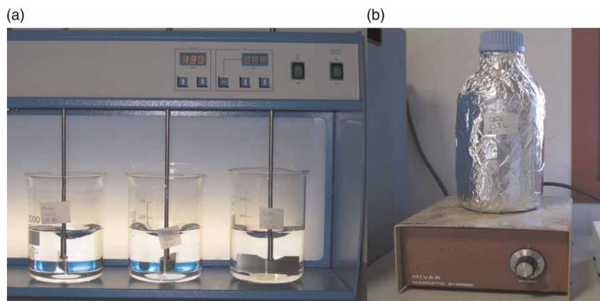
**Figure 1** | Oxidation test of MC-LR with sodium hypochlorite (a) and chlorine dioxide (b).
