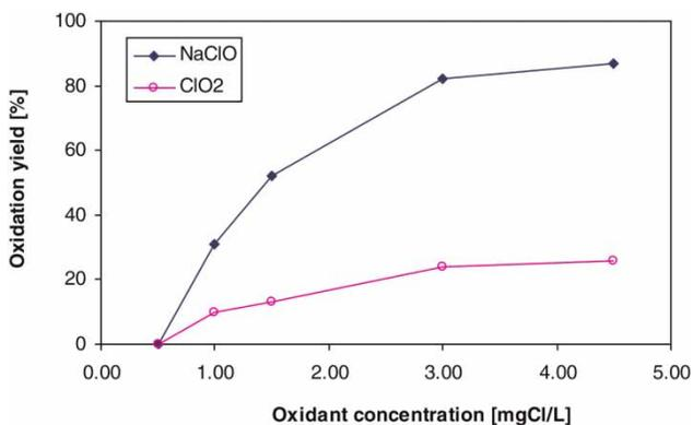
**Figure 2** | Oxidation yield of MC-LR at different sodium hypochlorite and chlorine dioxide concentration.
