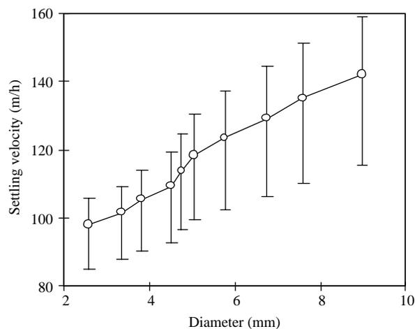
**Figure 4** Settling velocity of granules from G-SBR2
