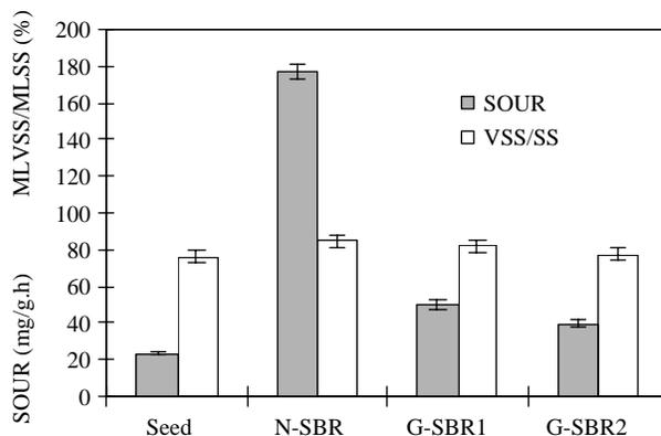
**Figure 8** SOUR of granules and sludge flocs after 112 days of cultivation
