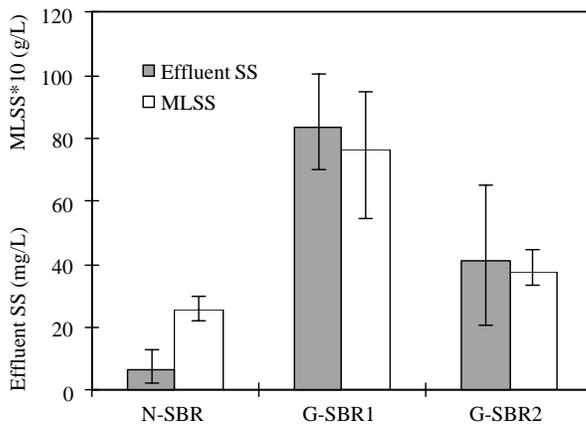
**Figure 6** Effluent suspended solid of reactors
