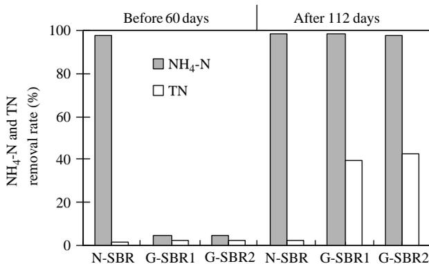
**Figure 10** Nitrification and denitrification of granules and sludge flocs
