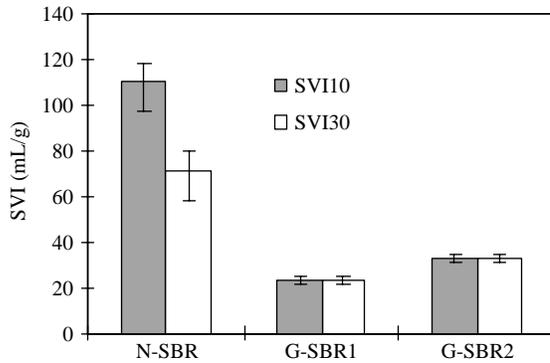
**Figure 5** SVI of granules and sludge flocs
