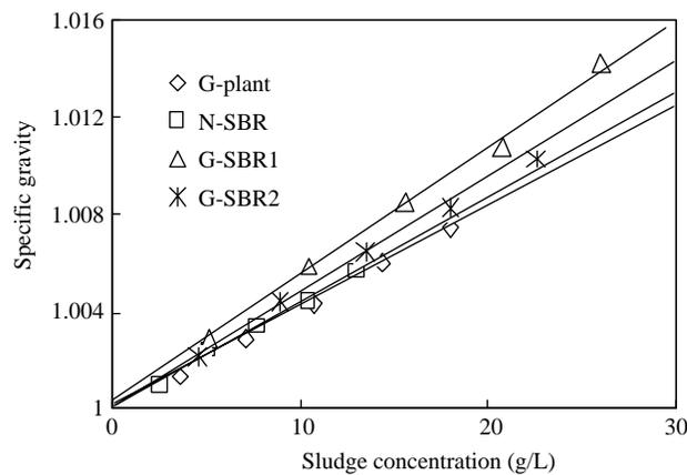
**Figure 3** Specific gravity of granules and sludge flocs
