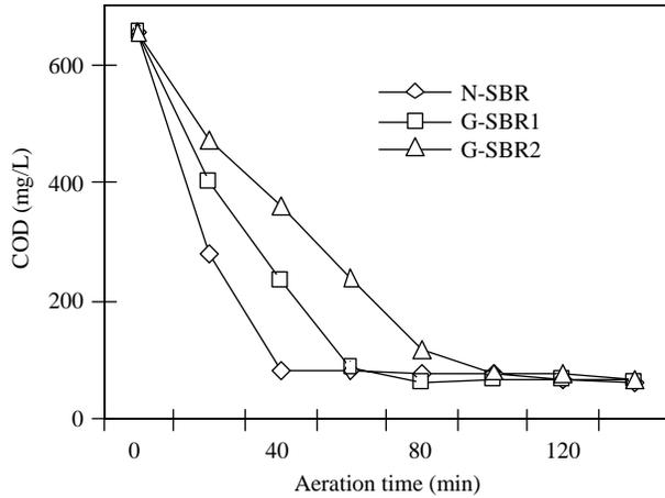
**Figure 9** COD removal of granules and sludge flocs
