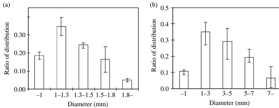
**Figure 2** Distribution of granule diameter (after 60 days) in (a) G-SBR1 and (b) G-SBR2
