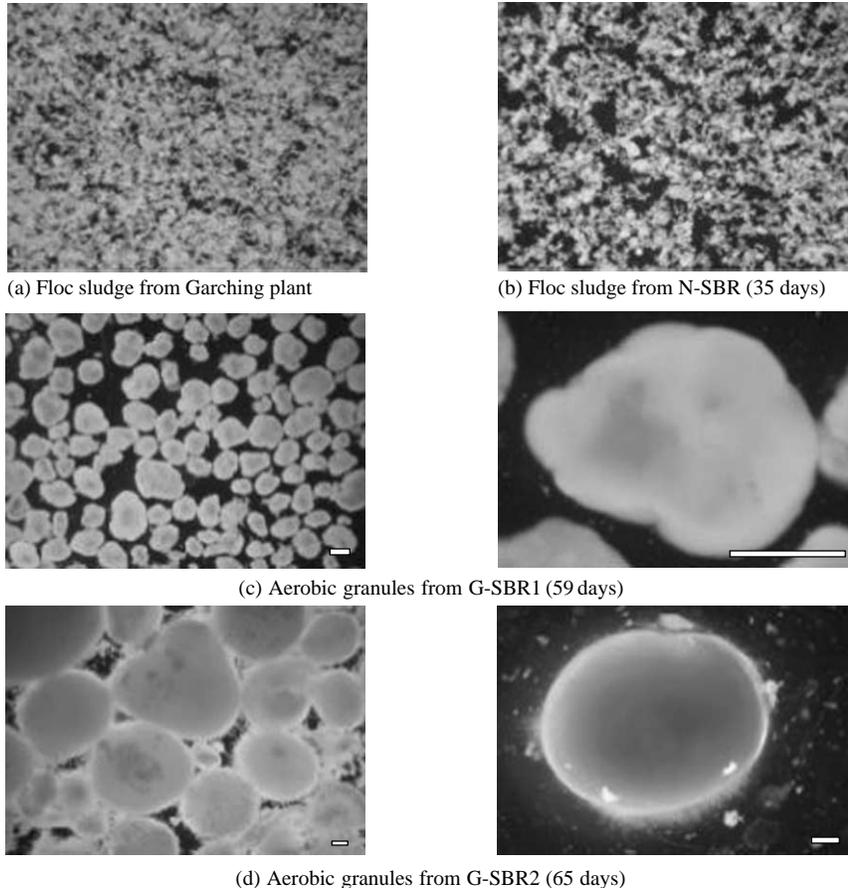
Figure 1 Microscopic examination of granules and sludge flocs (size of bar = 1 mm)
