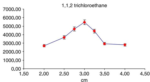
**Figure 1** | Results for the variation of the fibre position in the GC injector port for 1,1,2-trichloroethane. Numbers in the abscissa are centimetres while the ordinate are GC-ECD output, i.e. 'area counts'.
