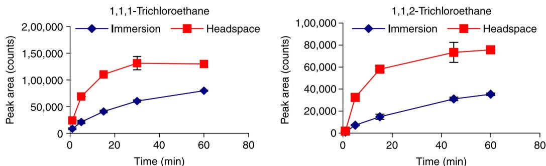
**Figure 3** | Optimization of the Fibre 2 extraction time for two chosen compounds (1,1,1-trichloroethane and 1,1,2-trichloroethane). Numbers in the abscissa are minutes while the ordinate are GC-ECD output, i.e. 'area counts'.
