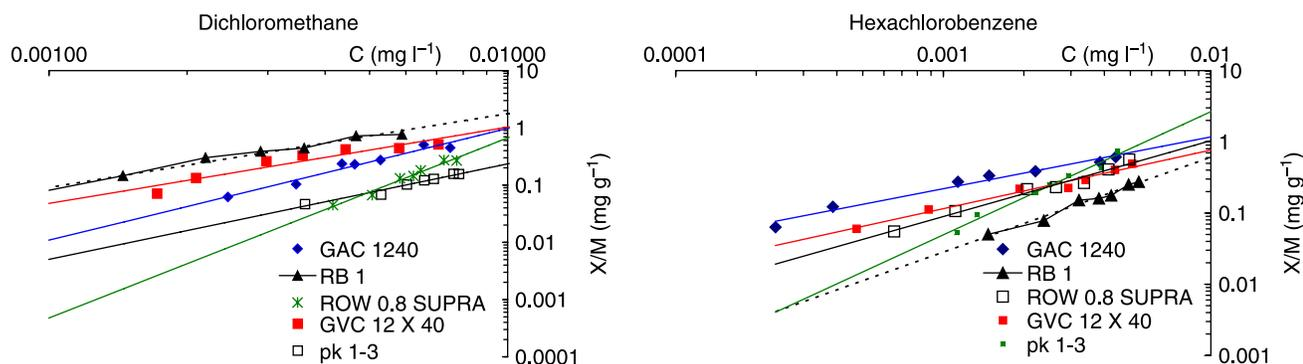
Figure 6 | Freundlich adsorption isotherms determined using SP $\mu$ E.
