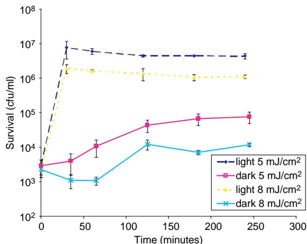
**Figure 1** | Repair of *E. coli* O157:H7 following LP UV irradiation at low doses of 5 and 8 mJ/cm<sup>2</sup>. Averages with standard deviations at 5 mJ/cm<sup>2</sup> are based on three separate experiments and at 8 mJ/cm<sup>2</sup> are based on five separate experiments.
