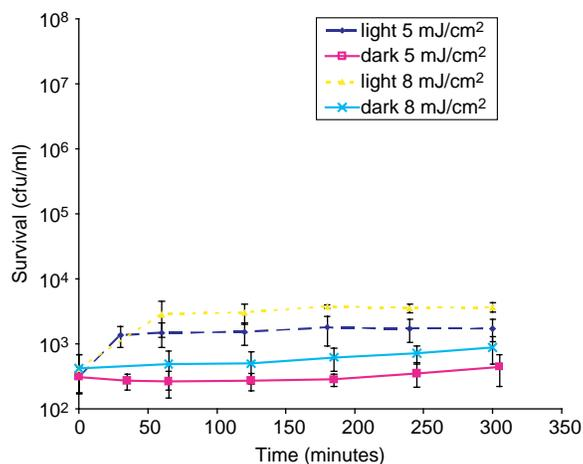
**Figure 3** | Repair potential of *E. coli* O157:H7 following MP UV irradiation at weighted doses of 5 and 8 mJ/cm<sup>2</sup>. Averages with standard deviations at 5 mJ/cm<sup>2</sup> are based on four separate experiments and at 8 mJ/cm<sup>2</sup> are based on three separate experiments.
