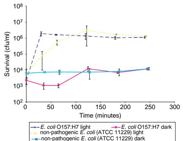
**Figure 2** | Comparison of repair potential between *E. coli* O157:H7 and non-pathogenic *E. coli* (ATCC 11229) following LP UV irradiation at 8 mJ/cm<sup>2</sup>. Averages with standard deviations are shown.
