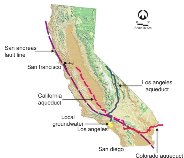
Figure 2 | California map showing major Los Angeles area water supply sources and the San Andreas Fault. The full colour version of all figures in this paper can be accessed by subscribers online at http://www.iwaponline.com/jws/toc.htm
