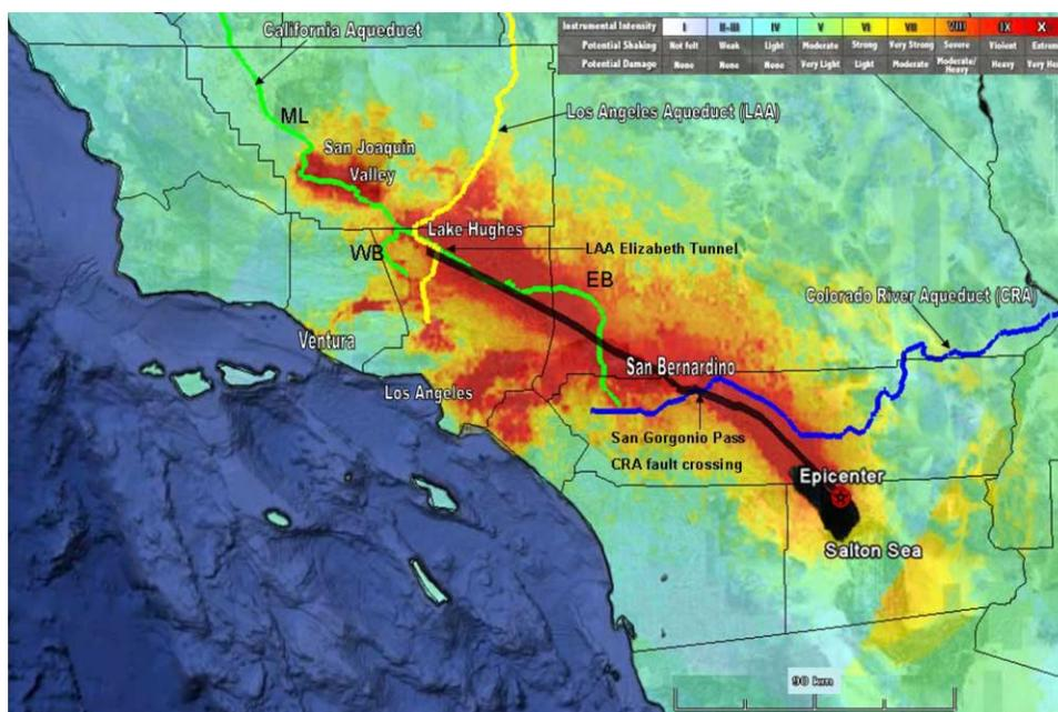
**Figure 1** | Southern California region showing the ShakeOut scenario epicentre (star), fault rupture (heavy line), shaking intensity (modified from USGS, 2010), Los Angeles Aqueduct (LAA), Colorado River Aqueduct (CRA), and California Aqueduct (ML, EB and WB are the California Aqueduct Main Line, East Branch and West Branch, respectively). The full colour version of all figures in this paper can be accessed by subscribers online at <http://www.iwaponline.com/jws/toc.htm>
