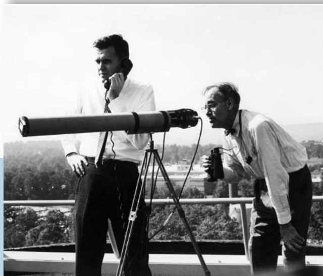
Figure 4. Sending a laser beam 25 miles from Crawford Hill, New Jersey (left) to Murray Hill (right) in 1960. At Crawford Hill, Robert Collins (left) aims a Bell Labs ruby laser at the top of the radar tower in Murray Hill as Willard Boyle prepares to fire it. Atop the tower in Murray Hill, Walter Bond (right) checks the alignment of the photomultiplier detector while Donald Nelson maintains phone contact with Crawford Hill.
