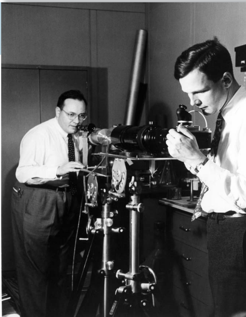
Figure 2. Arthur Schawlow and Geoffrey Garrett (right) aligning the Bell Labs ruby laser to obtain Fabry–Perot interference fringes for measuring the spectral linewidth of its output.
