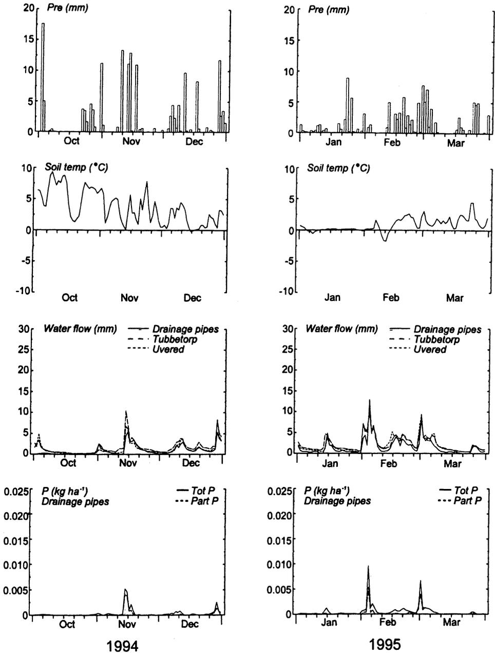
Fig. 7. Precipitation, soil temperature, waterflow and exports of total phosphorus (TotP) and particulate phosphorus (PartP) in drainage pipes, and in the streams of Uvered and Tubbetorp during Oct-Dec 1994 and Jan-Mar 1995.
