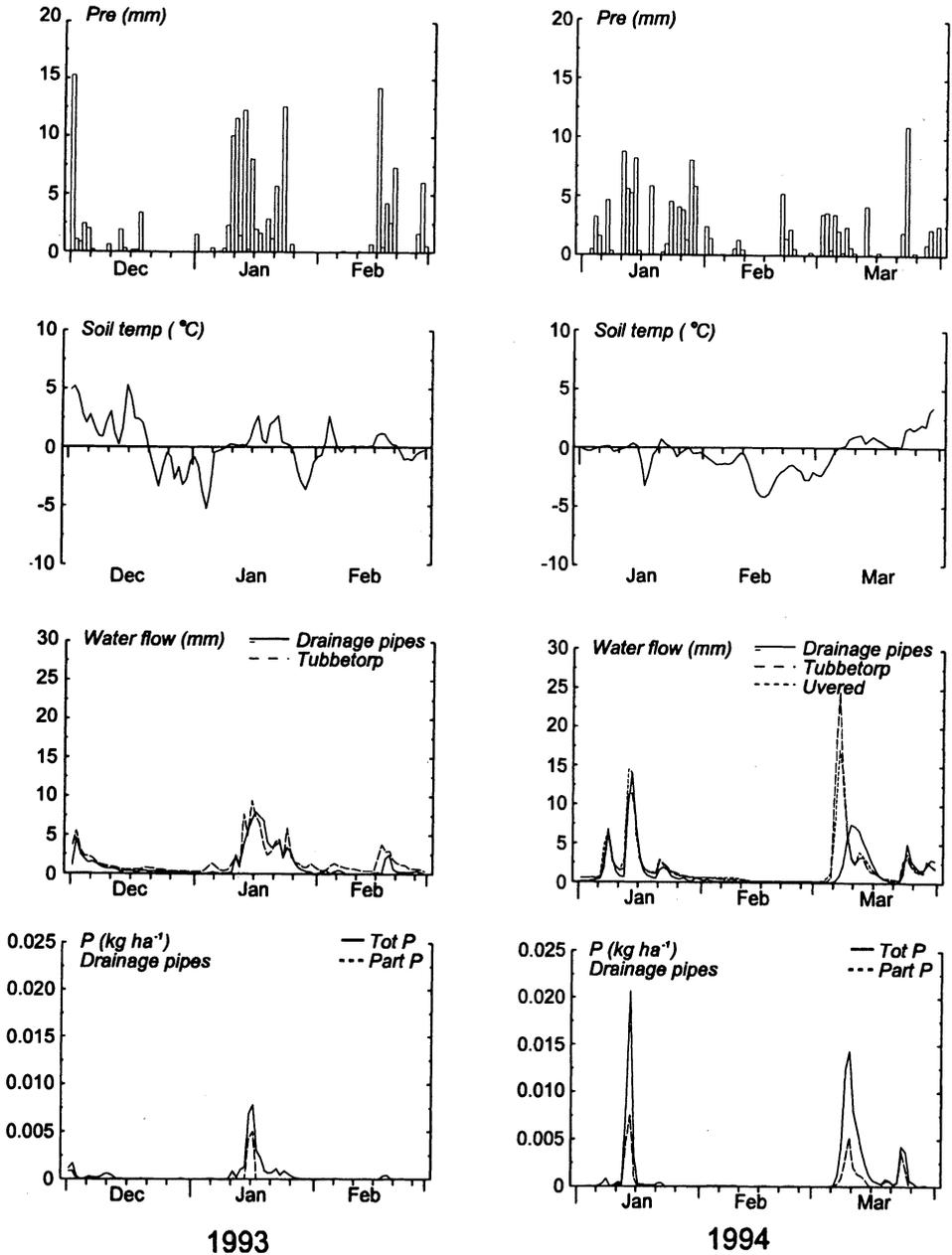
Fig. 6. Precipitation, soil temperature, waterflow and exports of total phosphorus (TotP) and particulate phosphorus (PartP) in drainage pipes, and in the streams of Uvered and Tubbetorp during Dec 1992-Feb 1993 and Jan-Mar 1994.
