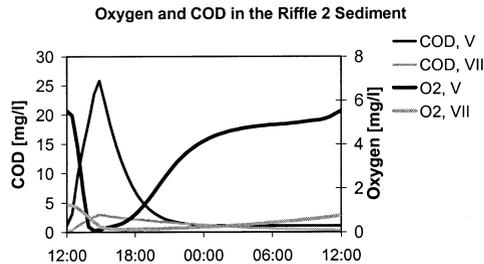
Figure 7 Sediment time series for COD and oxygen in riffle 2 for a hypothetical situation with a combined sewer overflow effluent (discharge of 2 m<sup>3</sup>/s with a duration of 2.4 h and a COD of 100 mg/l)
