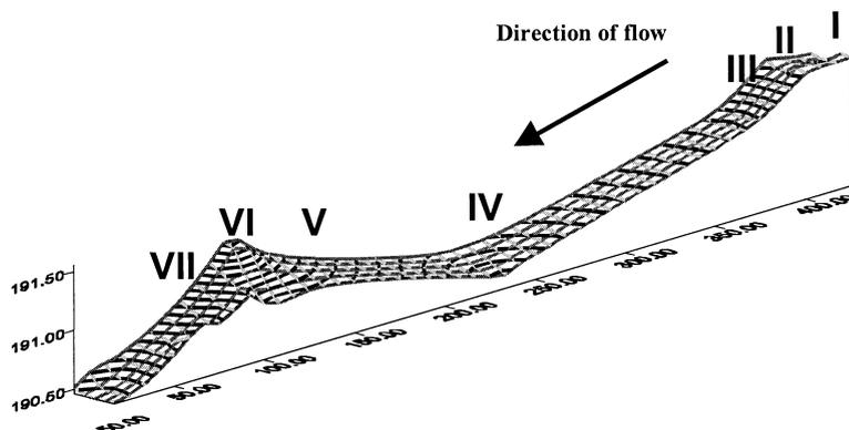
Figure 1 Longitudinal profile of the sediment surface with sampling cross-sections
