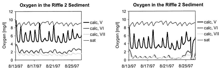
Figure 6 Sediment oxygen time series in riffle 2 (below the wastewater treatment plant effluent) for the August 1997 measuring campaign (left) and for a hypothetical situation with a wastewater treatment plant effluent with a COD of  $90 \text{ mg/l}$  instead of  $40 \text{ mg/l}$  (right)
