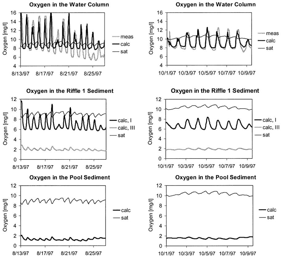
Figure 5 Oxygen time series in the water column (top), in the sediment of the pool (middle) and in the sediment of riffle 1 (bottom) for the August 1997 (left) and the October 1997 (right) measuring campaign. In the legends, "meas" means measured, "calc" means calculated, "sat" means saturation concentration in the water column, and "I" and "III" refer to the measurement cross-sections mentioned in the text (and shown in Figures 1 and 3)
