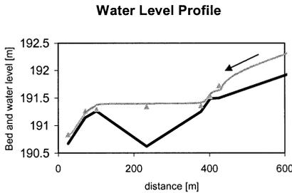
Figure 2 Level of the river bed (black line) and measured (grey markers) and calculated (grey line) water level in the study reach (left) and in part of the upstream, simplified reach (right)
