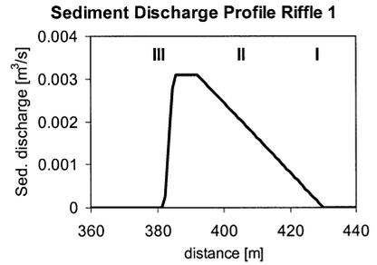
Figure 3 Sediment discharge in riffle 1. The maximum discharge was fitted with the aid of uranine data, the positions of in- and exfiltration zones (linearly in- or decreasing discharge) were fixed. The vertical lines mark the positions of the three measurement cross-section in the riffle
