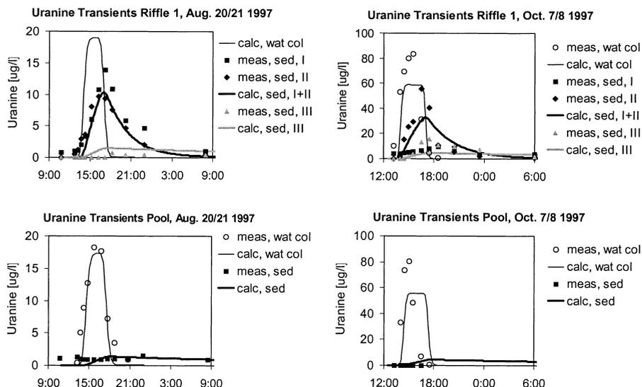
Figure 4 Measured (markers) and calculated (lines) tracer transients in riffle 1 (top) and in the pool (bottom) for the tracer experiment at August 20/21, 1997 (left) and at October 7/8, 1997 (right)
