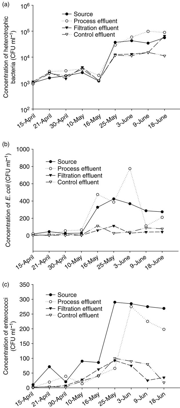
**Figure 1** | Levels of (a) heterotrophic bacteria, (b) *E. coli* and (c) enterococci as determined by plate count in the source water, process water, control water after filtration through aquifer material, and the final effluent after water has gone through the processor and filtration through aquifer sand material. All samples were taken from April to June 2004.
