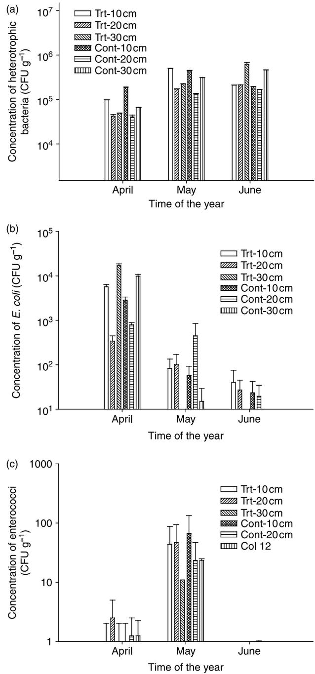
**Figure 2** | Concentrations of different bacterial groups from columns in aquifer materials after 15 d in the filtration tank: (a) heterotrophic plate counts, (b) *E. coli* concentrations and (c) enterococci plate counts.
