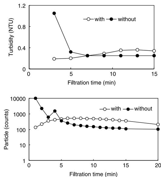
**Figure 3** Comparison of the filtrate turbidity and particles with and without underdrain
