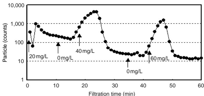
Figure 4 Particle count of the filtrate with a change in the coagulant dosage
