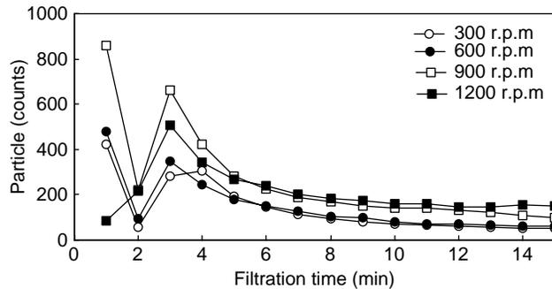
**Figure 6** Particle count of the filtrate with a change in mixing speed
