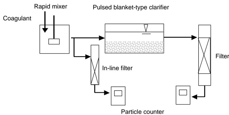
Figure 1 The pilot in-line filter and the pilot plant at Busan Water Quality Institute
