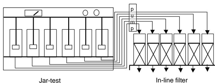
Figure 2 Test apparatus used to determine the coagulant dosage
