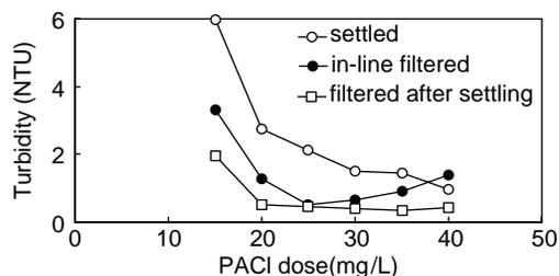
**Figure 8** Comparison of three water qualities for highly turbid water
