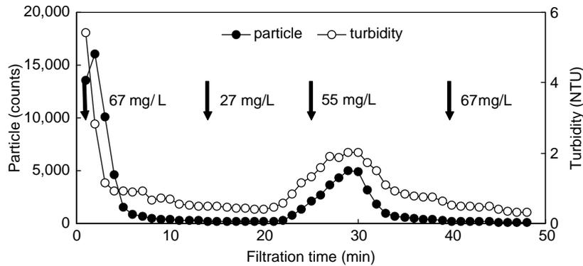
**Figure 5** Residual turbidity and particle count of the filtrate with a change in the coagulant dosage
