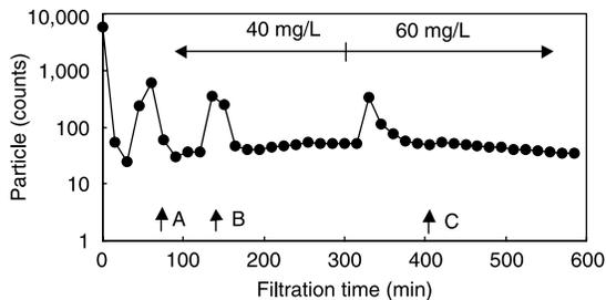
**Figure 7** Particle count of the filtrate with a change in coagulant dosing point and dosage
