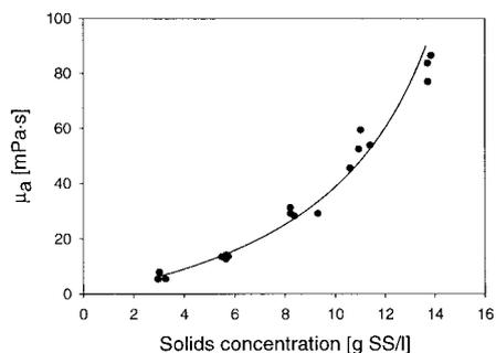
**Figure 5** Apparent viscosity for different activated sludge concentrations
