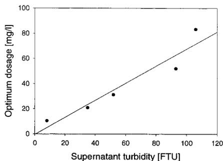
**Figure 4** Correlation between supernatant turbidity before conditioning and optimum polymer dosage ( $R^2=0.91$ ). The slope was  $6.8 \times 10^{-4}$  g/l/FTU, corresponding to 0.57 g Zetag 57 per g dispersed mass.
