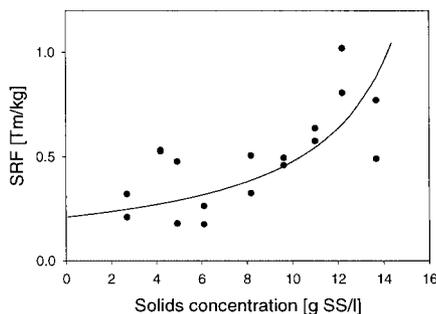
**Figure 8** Cake specific resistance to filtration for different activated sludge concentrations conditioned with 4.0 mg/g SS of Zetag 57
