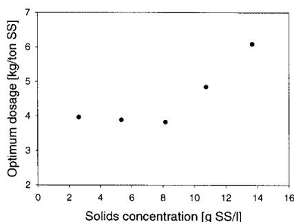
**Figure 2** Optimum polymer dosage per solids mass for different activated sludge concentrations
