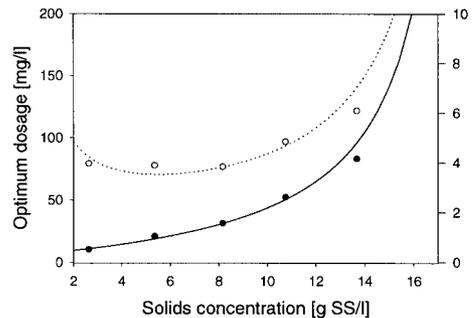
**Figure 10** Model calculation of the polymer demand in response to solids concentration for Åby activated sludge with  $m_{a,max} = 18.6$  g SS/l. (•): dosage per volume; (°): dosage per solids mass.
