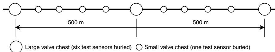
Figure 9 | Spots where test sensors were buried.
