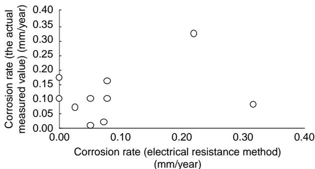
Figure 16 | Correlation between the electrical resistance method and the actual measured values.
