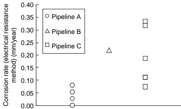
Figure 15 | Corrosion rates by the electrical resistance method.
