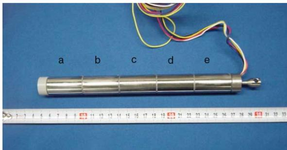
**Figure 7** | Segmented electrode.
