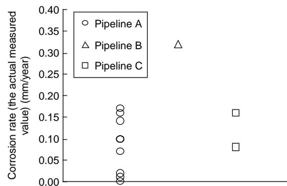
**Figure 14** | Corrosion rates based on the actual measured values.
