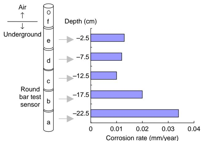
**Figure 13** | Relations between depth underground and corrosion rate (test site J).
