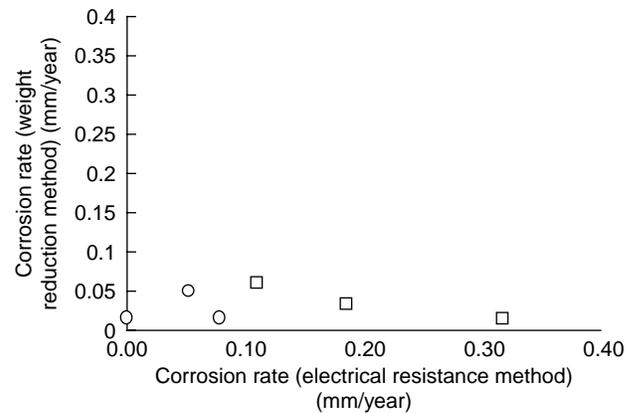
Figure 17 | Correlation between the electrical resistance method and weight reduction method.
