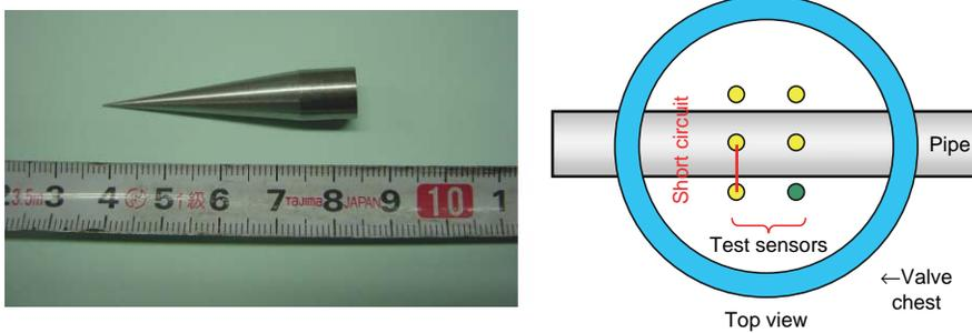
**Figure 4** | Chip-type test sensor.
