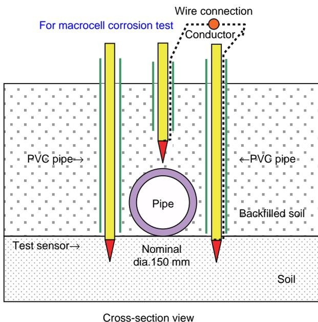
**Figure 5** | Buried test sensors.
