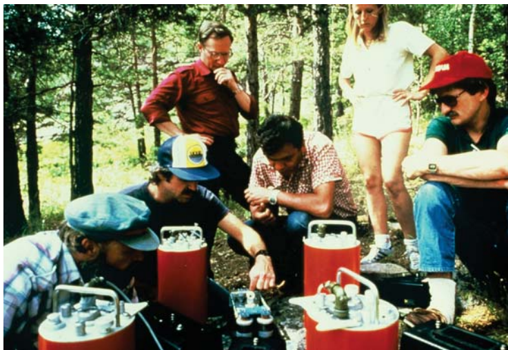
Figure 3. Monitoring a Soviet test site. A team of seismologists sponsored by the Natural Resources Defense Council, a nongovernmental American organization, setting up portable surface seismometers in July 1986 near the Soviet Semipalatinsk test site in Kazakhstan. Later, permanent seismometers were deployed in 100-m-deep boreholes. (Photo courtesy of NRDC.)
