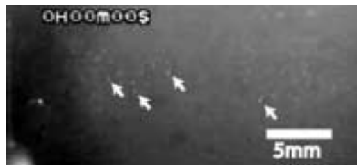
Fig. 3. Bubbles (white dots) created by IC at the beginning of the HIFU exposure (1.1 MHz, 0 sec.).
