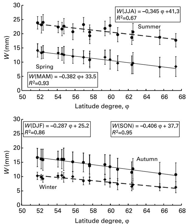
**Figure 2** Mean seasonal precipitable water as a function of geographical latitude,  $\varphi$ , 1989–2002. The error bar is the standard deviation between single monthly means and the mean seasonal value. Four linear equations between latitude and seasonal average precipitable water are given. Coefficient of determination,  $R^2$ , evaluates applicability of the linear formula
