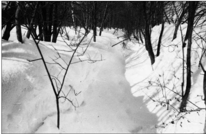
Figure 4 Snowdrifts formed in the Pakruostė-4 drain on 20 March 1996. The strips of woody vegetation on slopes resembled those in the openwork category: width of both strips approximated 3.0–3.5 m; height of trees averaged 5.4 m over the upper edges of the slopes; average stem density was 1.2 \text{ stems m}^{-2}
