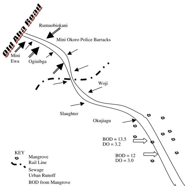
Figure 2 | A sketch of Amadi Creek showing the BOD, DO and Q of effluent discharged into it.
