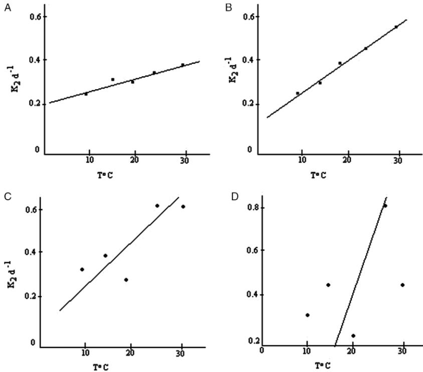
Figure 7 | Effect of temperature on  $k_2$  at the various stations A, B, C and D.
