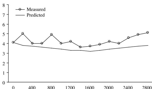
Figure 9 | Predicted and measured oxygen sag curve for Amadi Creek.
