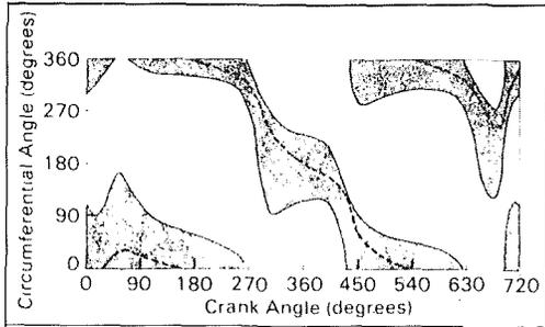
Fig. 12 Pressure curve extent plot for the bearing as obtained from the new curve fit (partial extent).
