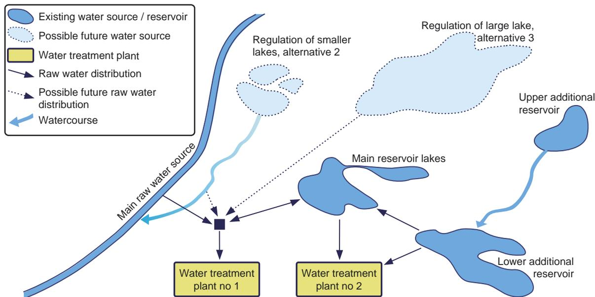
**Figure 1** | Schematic description of the Gothenburg raw water system. Possible future raw water supplies included in the analysis are further described in the *Risk-reduction alternatives* section.
