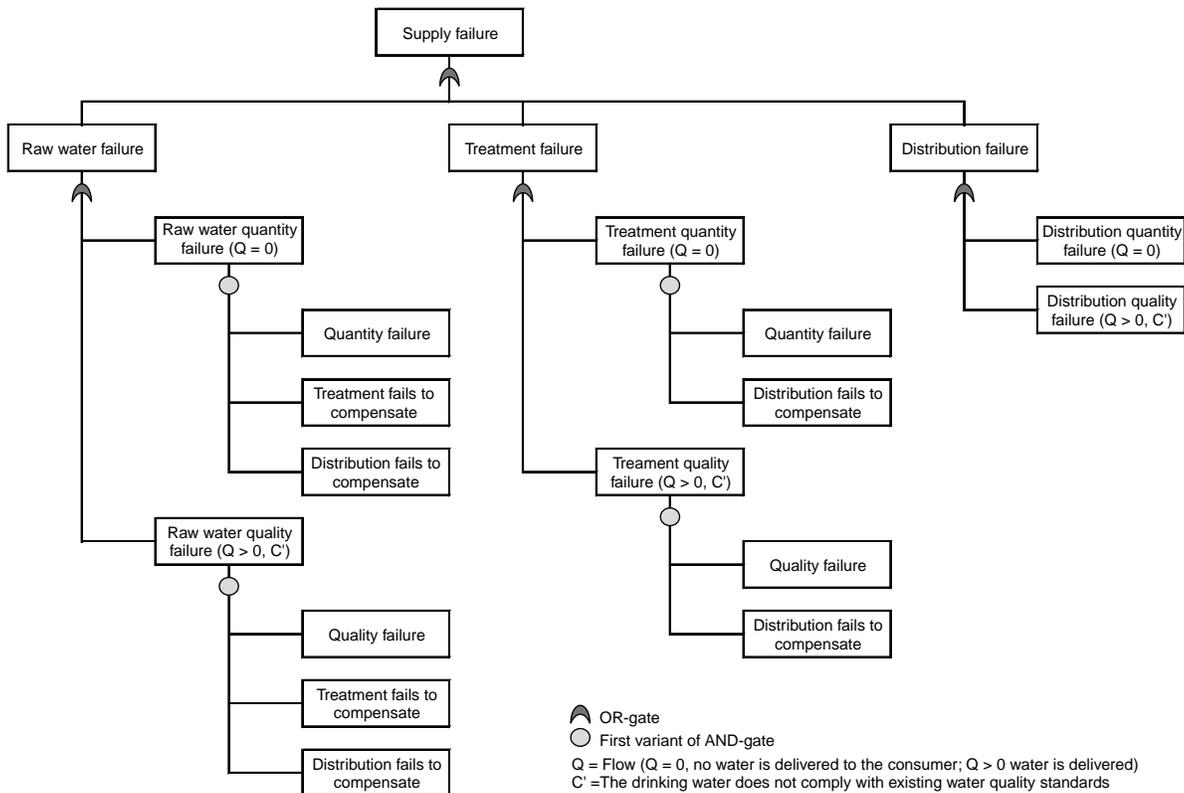
Figure 3 | Schematic fault tree including the main type of events.
